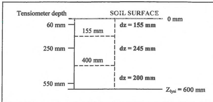
Figure 2-9 : Calculation of the difference of depth between the tensiometers
