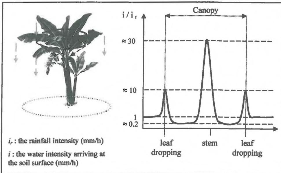
**Figure 1-4 : Heterogeneity of the rainfall intensity arriving at the soil surface of a banana plantation**
