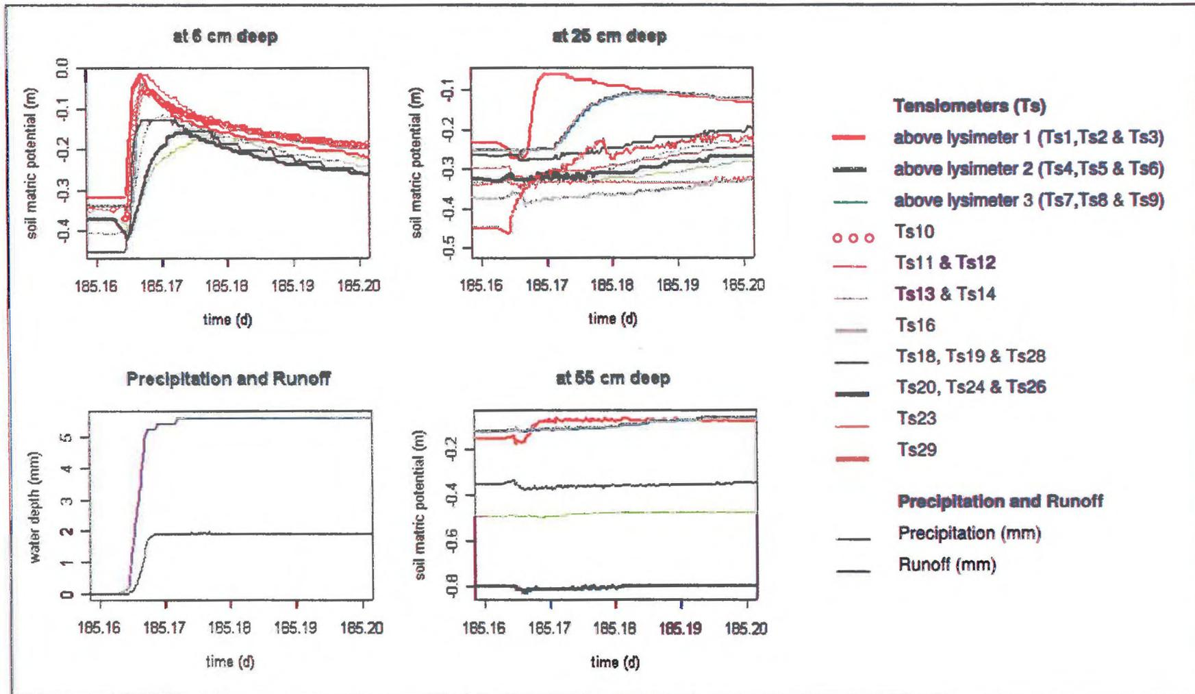
Evolution of each tensiometer according its depth during Event 1
