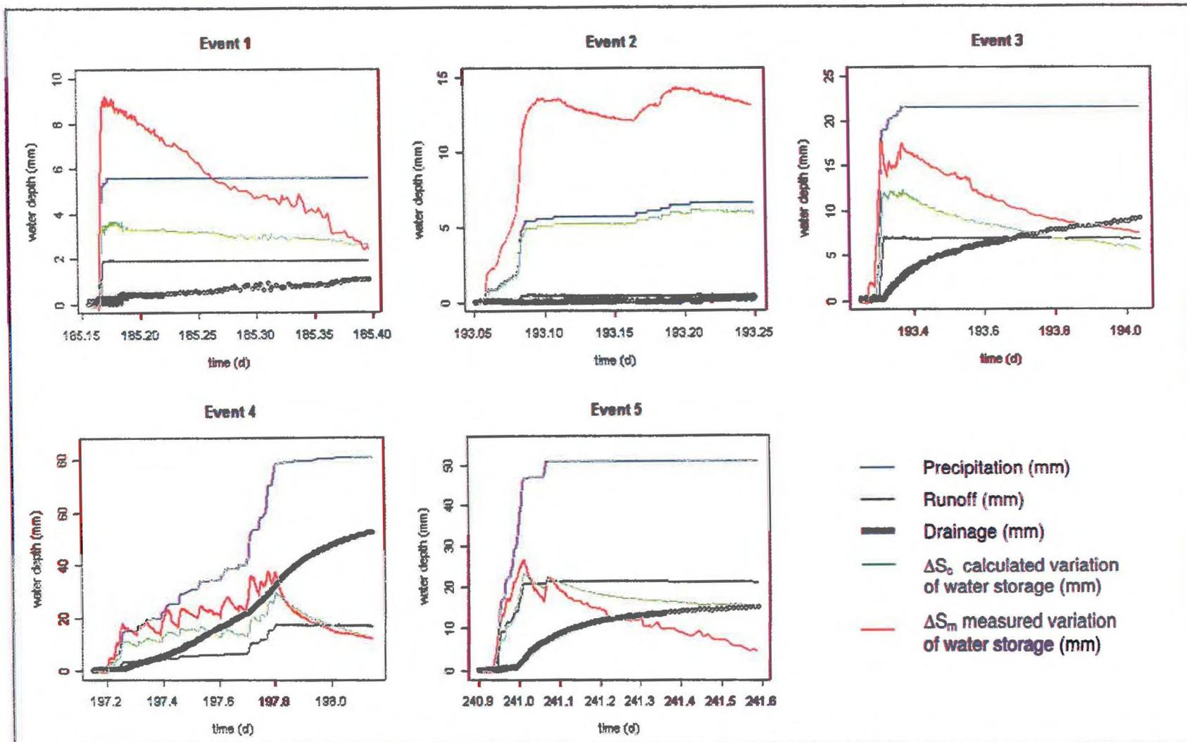
Figure 3-5 : Evolution of the runoff, drainage and water storage during the rain events
