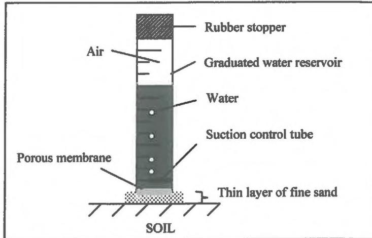
Figure 2-3 : Schematic diagram of the Decagon tension disc infiltrometer
