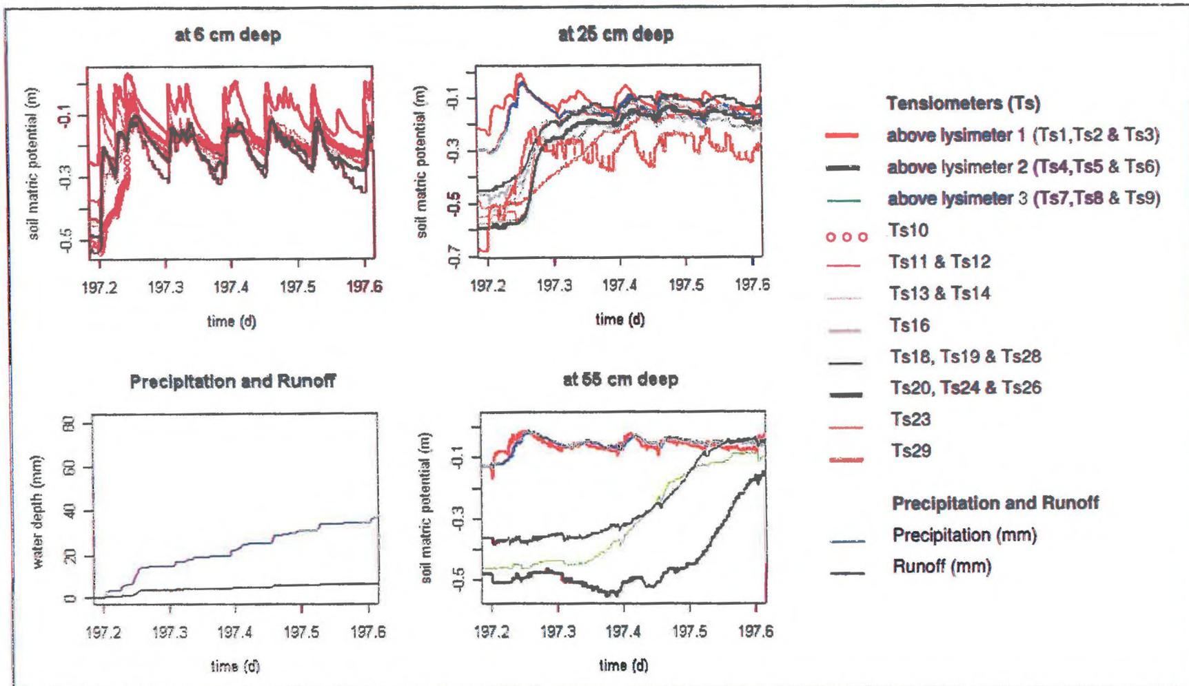
Evolution of each tensiometer according its depth during Event 4
