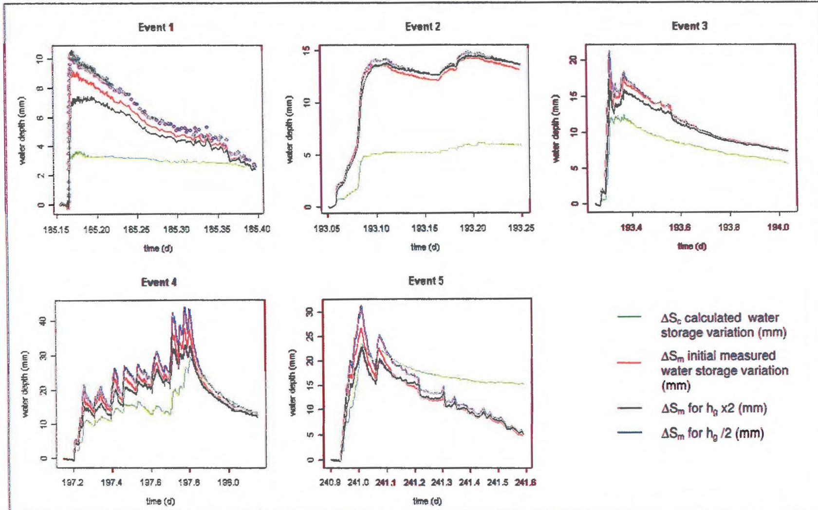
Effect of the variation of the scale parameter for the water pressure  $h_0$  (m)
