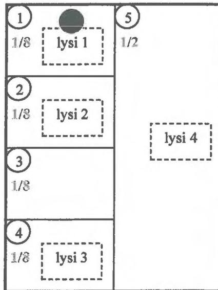
**Figure 2-8 : Division of the plot in subplot to estimate the drained water volume**
