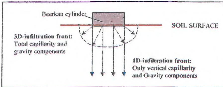
Figure 3-2 : Explanation of the difference between 1D and 3D analyses of data
