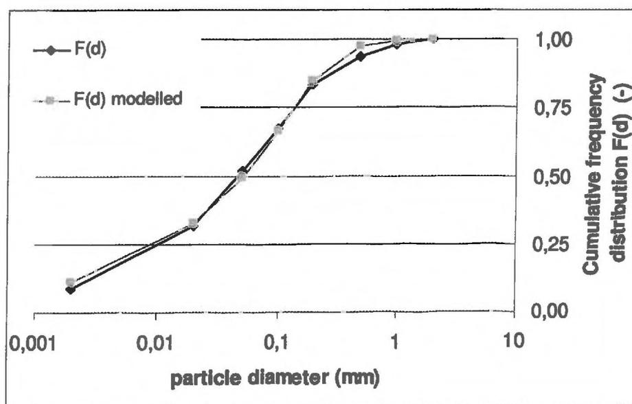
Figure 3-1 : Experimental and modelled particle size distribution curve of surface soil
