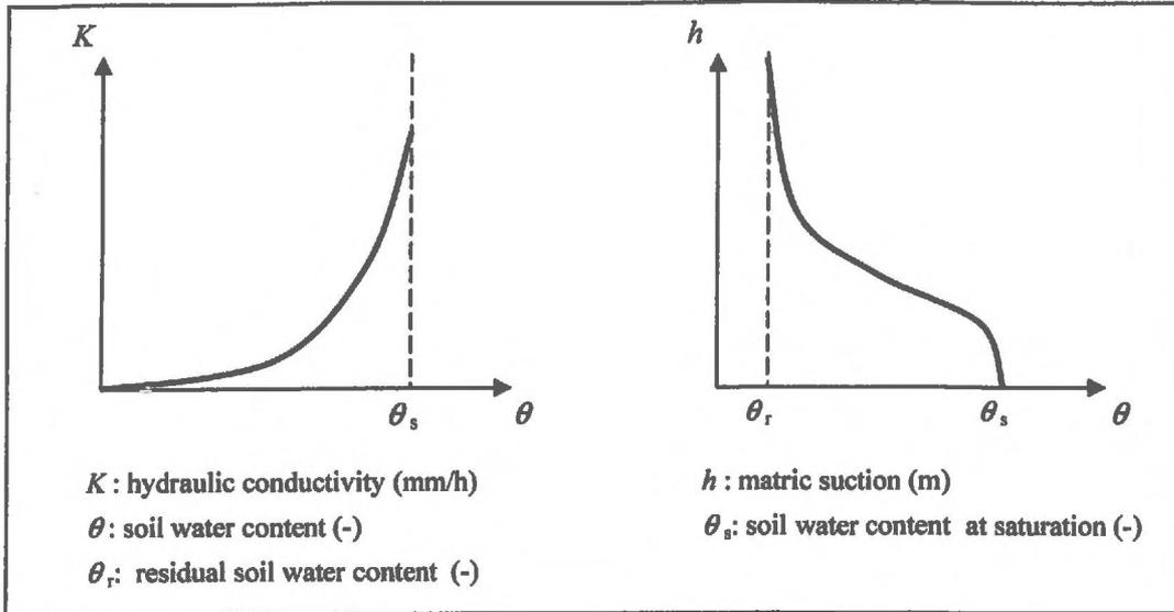
An example of hydraulic conductivity and water retention curves
