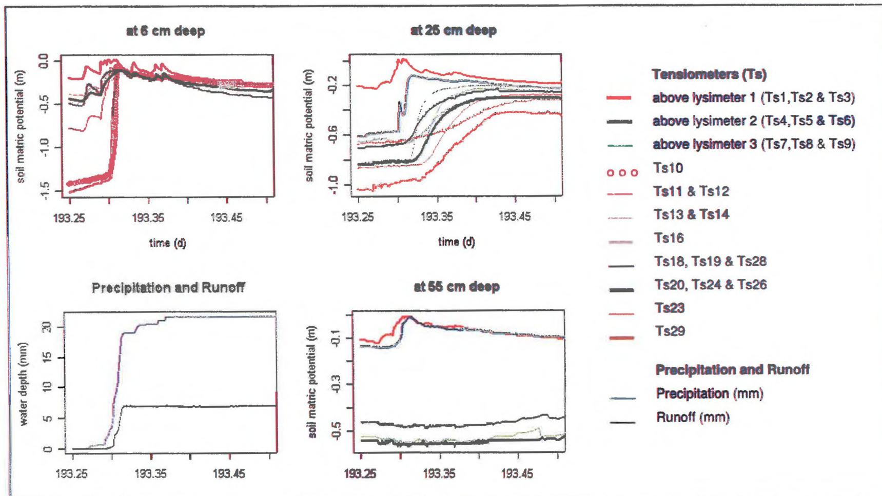
Evolution of each tensiometer according its depth during Event 3
