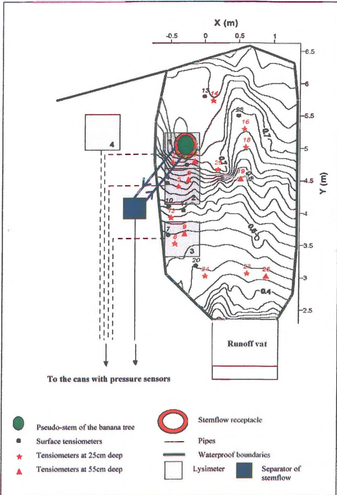
**Figure 2-6 : Plot layout for banana hydrology experiment in Guadeloupe**
