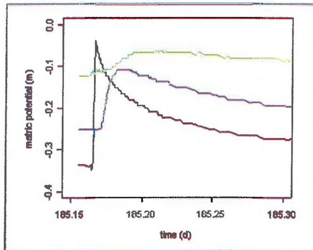
**Figure 3-8 : Typical variation of the soil matric potential at 6 (black line), 25 (blue line) and 55 cm deep (green line) during a rainfall event**
