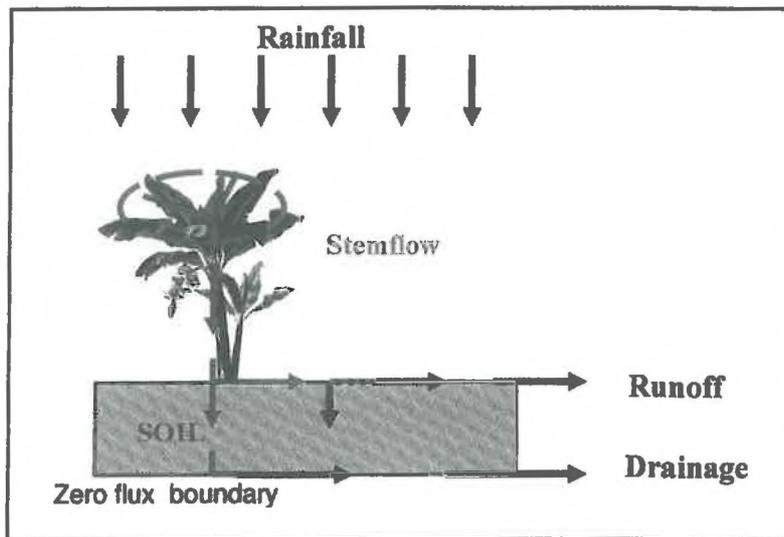
Figure 2-7 : Scheme of the water balance at the plot scale
