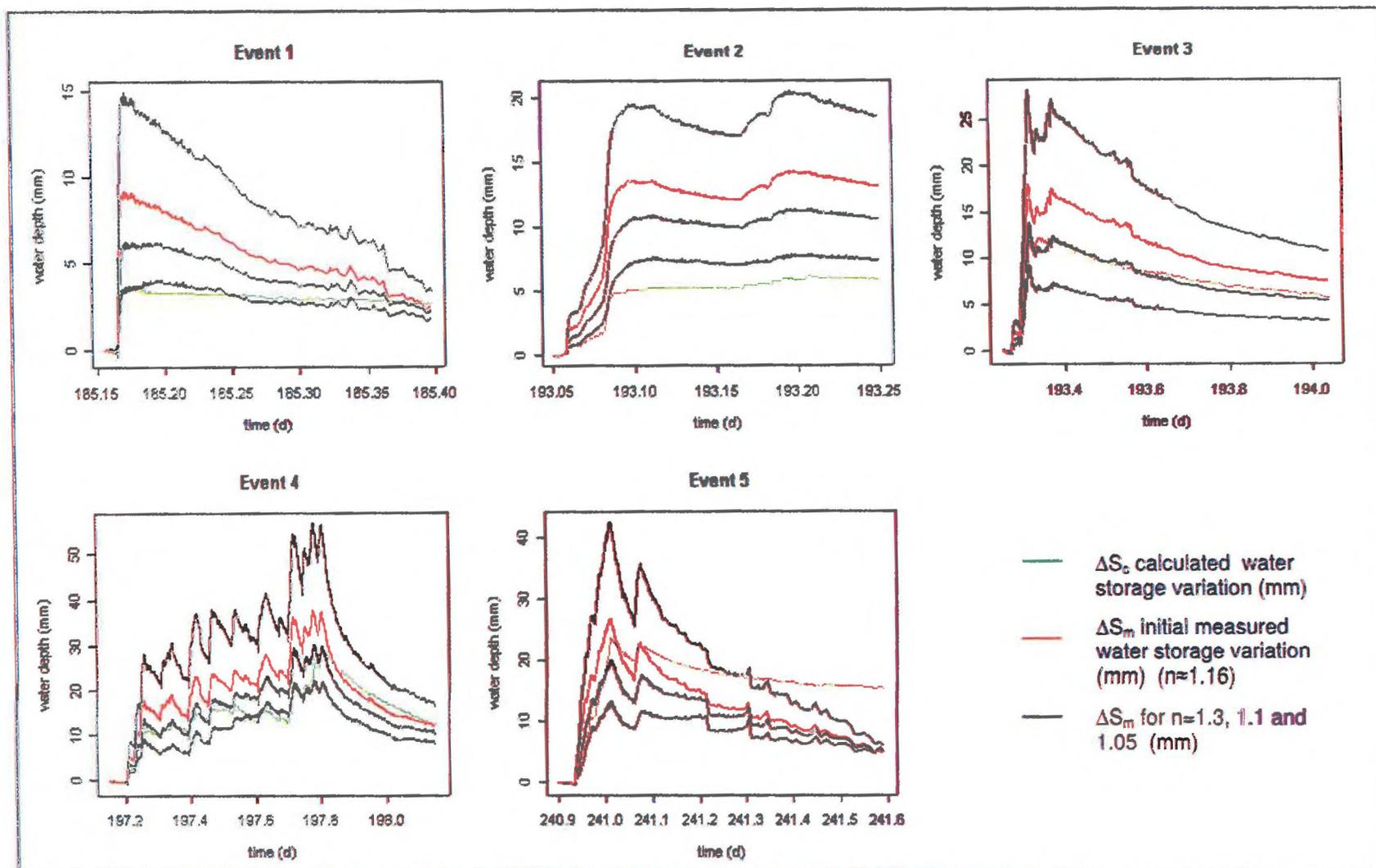
Effect of the variation of the shape parameter for the water retention curve  $n$
