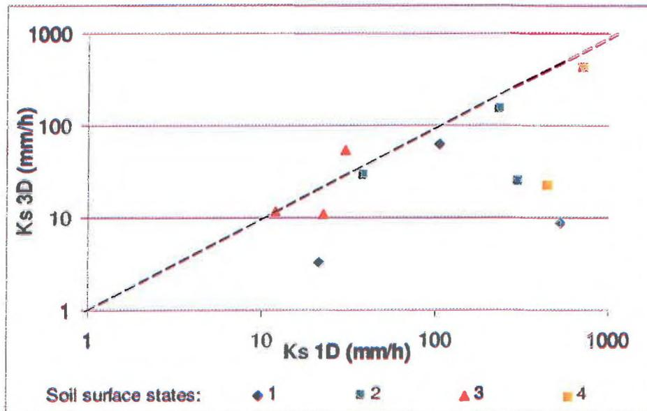
Figure 3-3 : Comparison between 1D and 3D hydraulic conductivities at saturation
