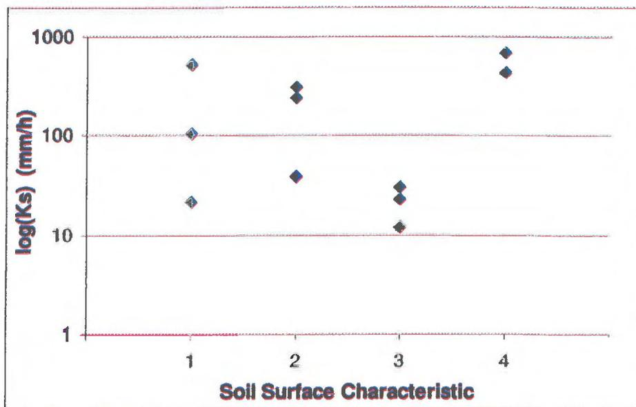
**Figure 3-4 : Characterisation of the hydraulic conductivity of the soil surface using the Beerkan method in one-dimension.**
