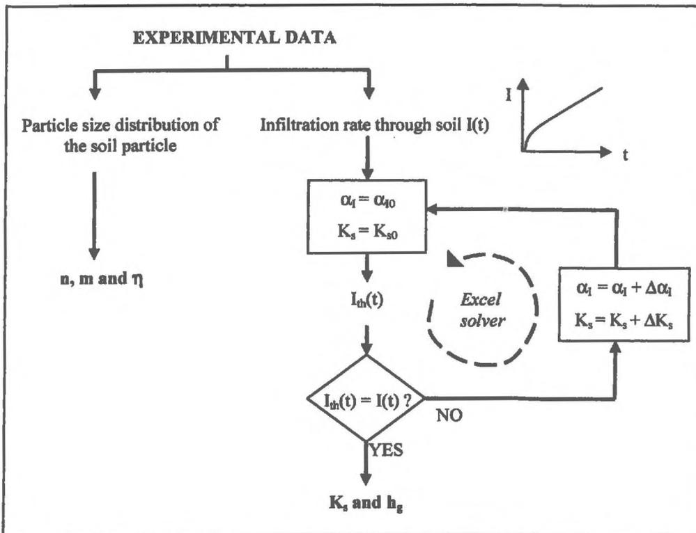
Figure 2-2 : Algorithm describing the calculations when analysing the Beerkan data
