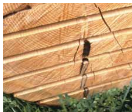
40. The absence of pruning leaves knots that decrease the timber quality (here: a branch that created a non-adherent knot in the most external planks).
