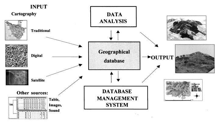
Fig. 1. General structure of a GIS.
