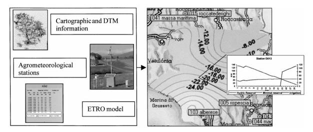
Fig. 4. Water deficit of the Grosseto lowland (26 June 1997) as estimated by ETRO. In input the different informative layers and in output the cartographic representation.
