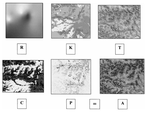
Fig. 11. Information layers for RUSLE model  $(T=L\times S)$ .
