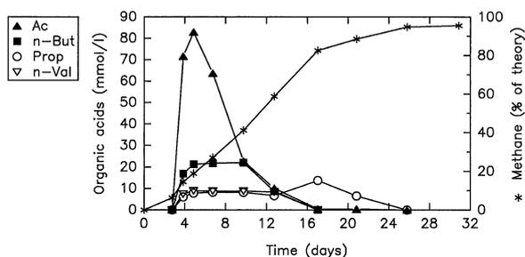
Figure 5. Methane production (\*) and formation of organic acids by an anaerobic sludge culture (0.25% VSS) during fermentation of 1% PHBV (8.4% HV) at 35 °C and pH 7.2.
