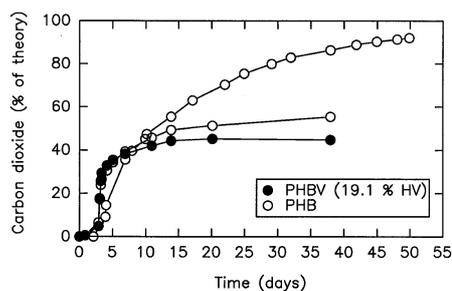
Figure 3. Carbon dioxide production observed during three degradation experiments with 0.1% PHB and 0.1% PHBV (19.1% HV) using a modified Anaerobic Sturm-test as degradation test apparatus (0.025% VSS).
