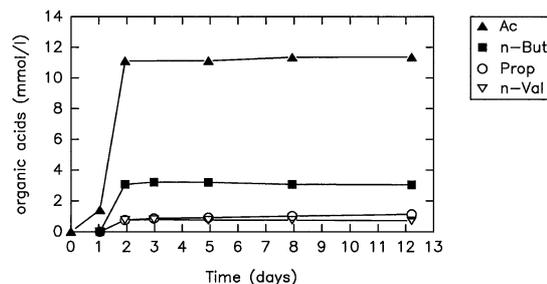
Figure 4. Accumulation of organic acids by a selective culture during fermentation of 0.1% PHBV (8.4% HV) at  $35^\circ\text{C}$  and  $\text{pH } 7.2$ .
