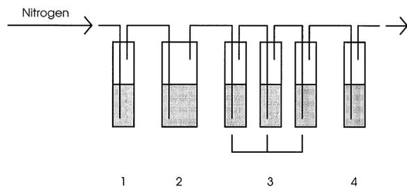
Figure 1. Scheme of degradation test apparatus with carbon dioxide measuring (Anaerobic Sturm-test).
