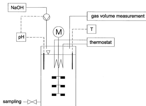
Figure 2. 6 l stirred tank reactor with pH control, temperature control, and gas metering for the fermentations with quantitative biogas determination (T: thermometer, M: stirring motor).
