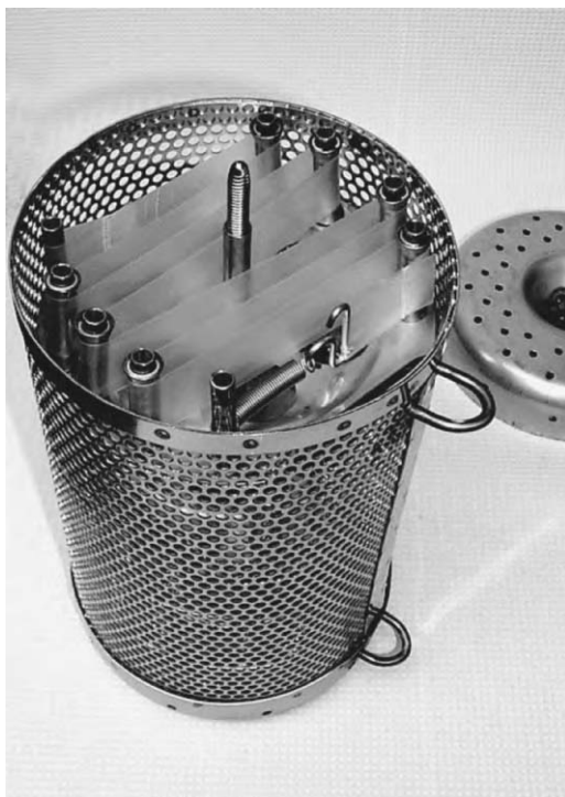
FIGURE 4.3 A commercially available stainless steel deployment canister (see Section 4.7), which has a capacity of five 1-mL triolein SPMDs. Each SPMD is placed on a separate deployment rack and the five deployment racks are held in place by a threaded center pin.
