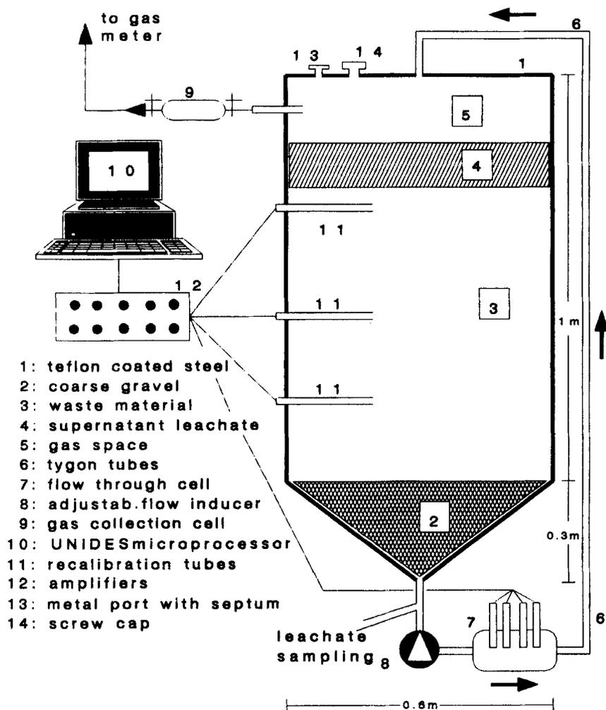
Fig. 1: Scheme of experimental reactor (steel version)
