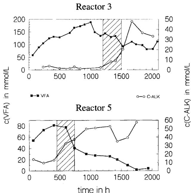
**Fig. 4:** Concentration of volatile fatty acids (VFA) as a function of time. VFA accumulate during acidogenesis in the reactor. Switching into methanogenesis leads to an increase of the pH (hatched area) and a subsequent increase in carbonate alkalinity (C-ALK).
