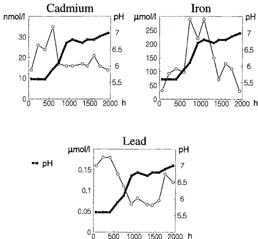
**Fig. 2:** Total dissolved metal concentration and pH plotted as a function of time for reactor 5
