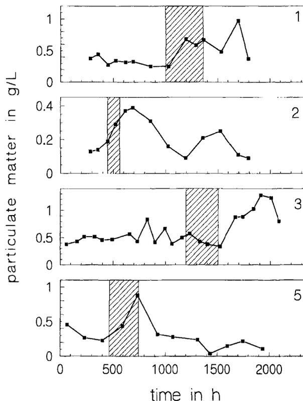
Fig. 7: Change of particulate matter content of the leachate with time in all reactor experiments. The hatched area denotes the increase of the pH during the anaerobic digestion process. The numbers in the upper right corner of each plot refer to the reactor.
