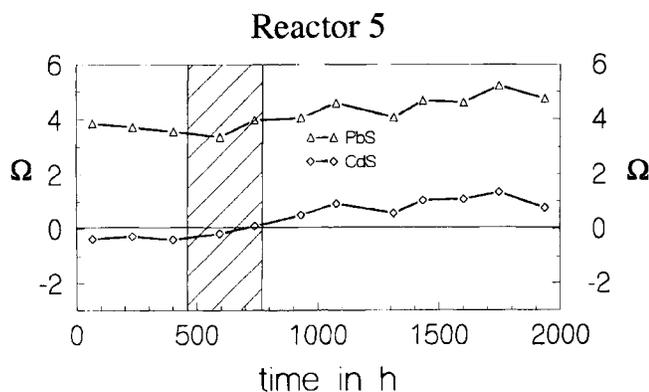
**Fig. 5:** Saturation indices  $\Omega$  for PbS and CdS plotted as a function of time
