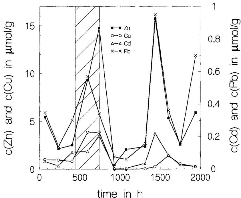
**Fig. 8:** Trace metal content of the particulate matter from the leachate of reactor 5 as a function of time
