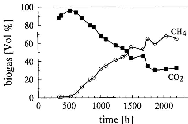
**Fig. 3:** The relative gas composition measured in reactor 3 as a function of time. It clearly indicates the change from acidogenesis to methanogenesis
