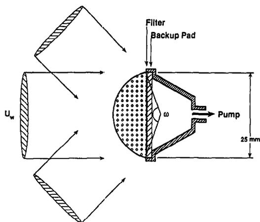
Fig. 1. Schematic diagram of the new aerosol sampler with multi-directional sampling capability.
