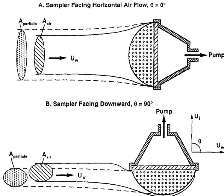
Fig. 3. Schematic representation of the limiting streamlines and particle trajectories for the two inlet orientations.
