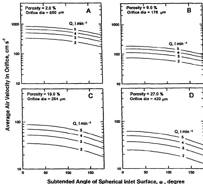
Fig. 2. Calculated air velocities in evenly spread circular orifice in a spherical inlet surface, filter diameter = 25 mm.
