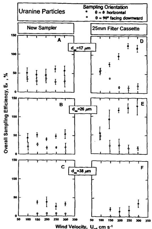
Fig. 4. Wind-tunnel data of the overall sampling efficiencies for the new sampler and the closed-face 25 mm filter cassette.
