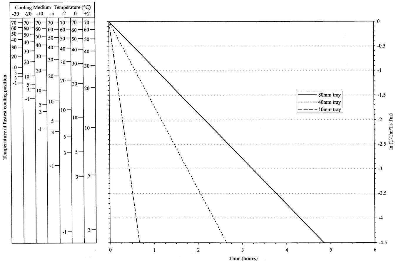
Fig. 4. Cooling time prediction graph for the bottom surface (fastest cooling position) under the low flow regime.
