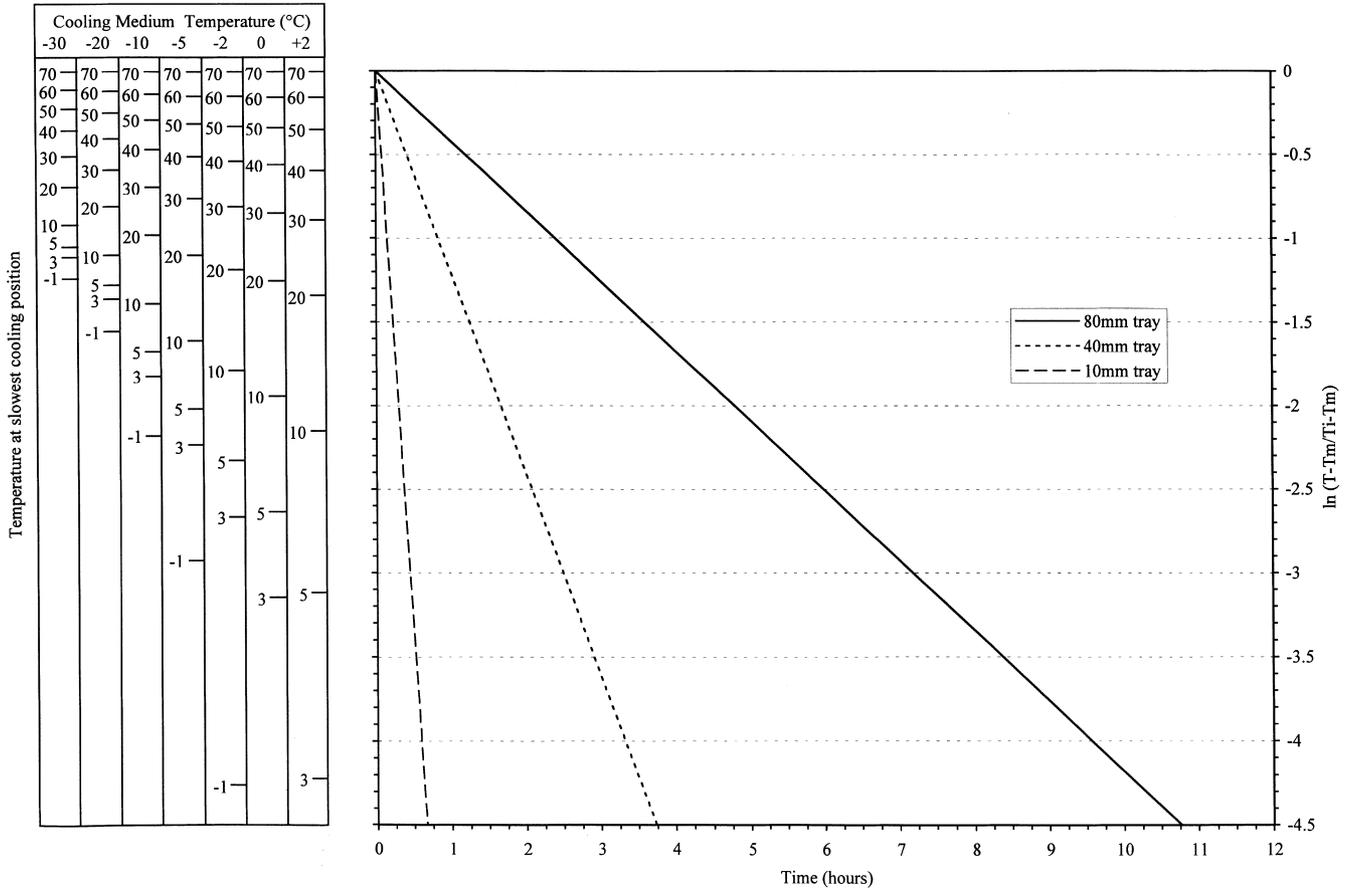
Fig. 3. Cooling time prediction graph for the slowest cooling position under the high flow regime.
