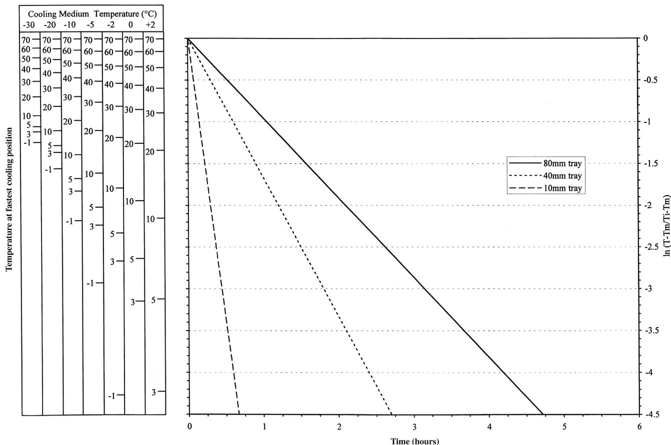
Fig. 5. Cooling time prediction graph for the bottom surface (fastest cooling position) under the high flow regime.
