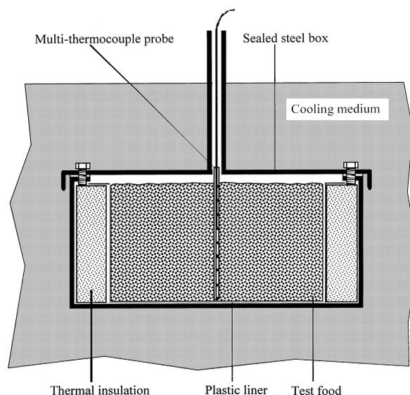
Fig. 1. Cross section of the sealed, lidded trays used in the immersion experiments (not to scale).
