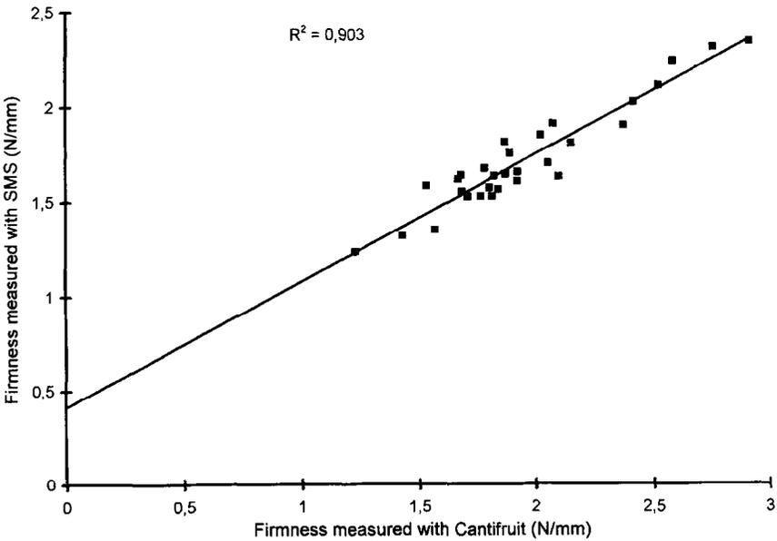
Fig. 6. Comparison of firmness measured with the *Cantifruit* and the SMS, 12 days after picking.
