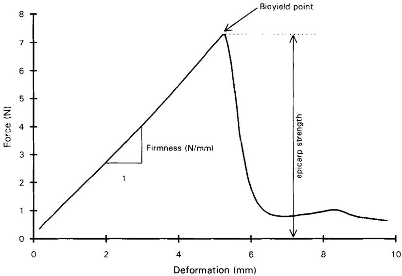
Fig. 3. Typical force–deformation curve obtained with the SMS universal testing machine during penetration of individual tomato.
