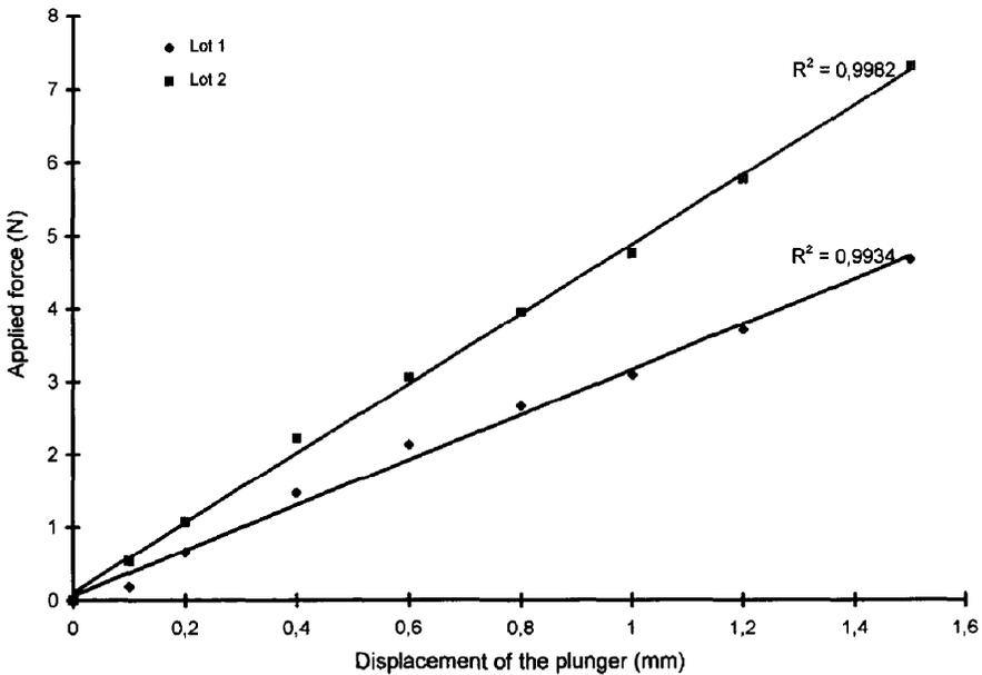
Fig. 4. Force–deformation relationship for two tomatoes, one day after picking.
