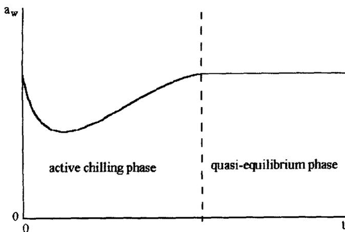
Fig. 1. Concept diagram showing the change in  $a_w$  during a typical chilling experiment in which the internal water movement rate within the product cannot maintain a fully wetted product surface.
