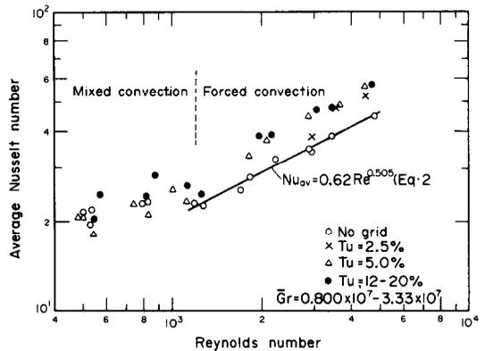
FIG. 9. Variation of average Nusselt number as a function of Reynolds number with turbulence intensity as parameter.
