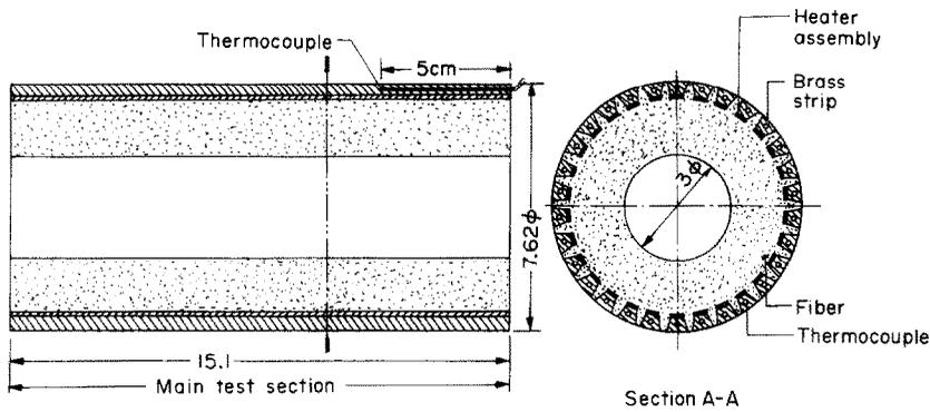
FIG. 1. Details of the test cylinder (all dimensions in cm).
