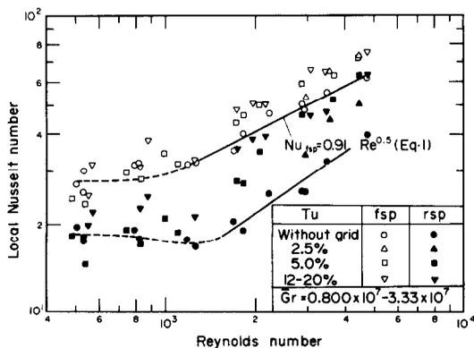
FIG. 8. Variation of local Nusselt number at fsp and rsp as a function of Reynolds number with turbulence intensity as parameter.
