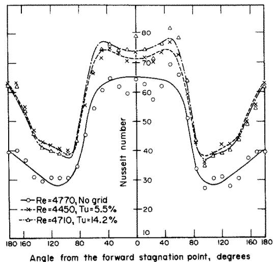
FIG. 5. Influence of turbulence intensity on local Nusselt number in forced convection ( $Re \approx 4700$ ).
