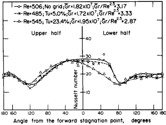
FIG. 6. Influence of turbulence intensity on local Nusselt number in mixed convection ( $Re \approx 500$ ).
