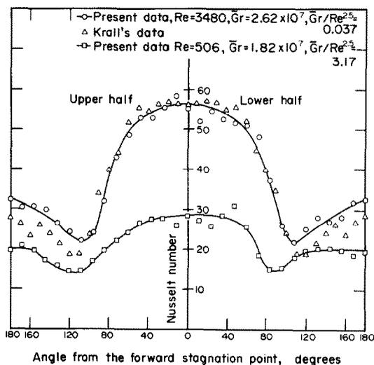
FIG. 2. Typical distribution of local Nusselt number in (i) forced convection,  $Re = 3480$  and (ii) mixed convection  $Re = 506$ .
