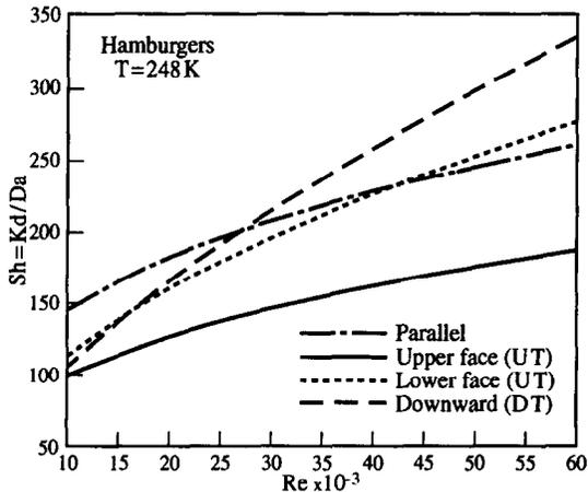
Fig. 6. Predicted variation of  $Sh$  with  $Re$  for hamburgers at  $T_a = 248$  K and for different types of air flow.
