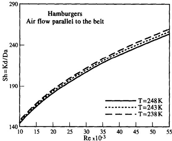
Fig. 4. Predicted variation of  $Sh$  with  $Re$  for hamburgers at different air temperatures and for air flow parallel to the belt.
