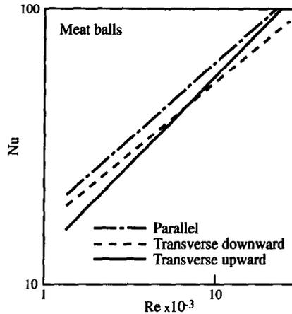
Fig. 2. Regression curves of  $Nu$  vs  $Re$  for meat balls in belt freezers for different types of air flow, at  $T_a = 248$  K.
