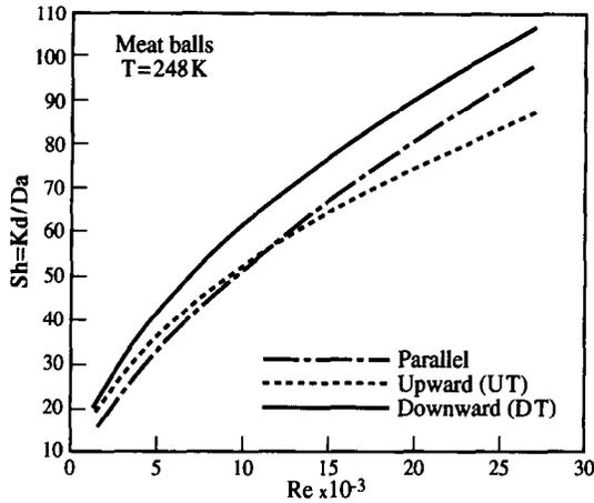
Fig. 5. Predicted variation of  $Sh$  with  $Re$  for meat balls at  $T_a = 248$  K and for different types of air flow.
