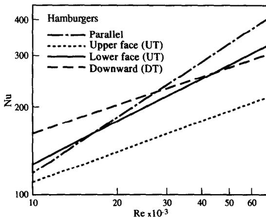
Fig. 1. Regression curves of  $Nu$  vs  $Re$  for hamburgers in belt freezers for different types of air flow, at  $T_a = 248$  K.
