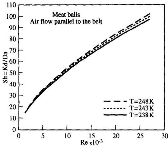
Fig. 3. Predicted variation of  $Sh$  with  $Re$  for meat balls at different air temperatures and for air flow parallel to the belt.
