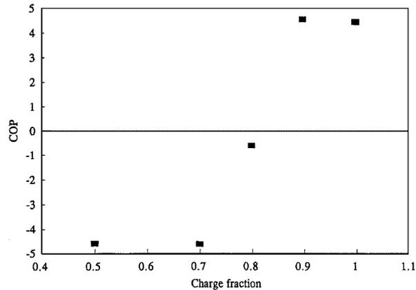
Figure 8. Coefficient of performance versus charge fraction.
