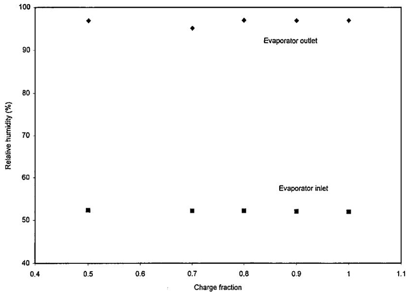
Figure 5. Relative humidity of air at the evaporator versus charge fraction.
