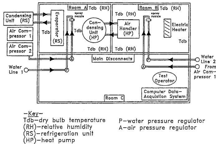
Figure 1. Schematic diagram of the air conditioning test facility.
