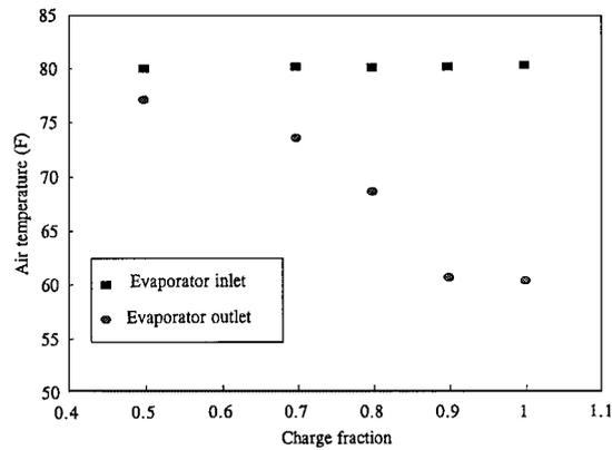
Figure 4. Air temperature at the evaporator versus charge fraction.
