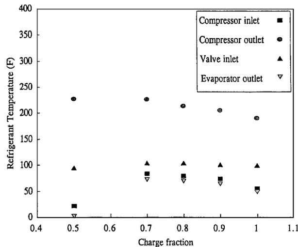
Figure 2. Refrigerant temperature versus charge fraction.
