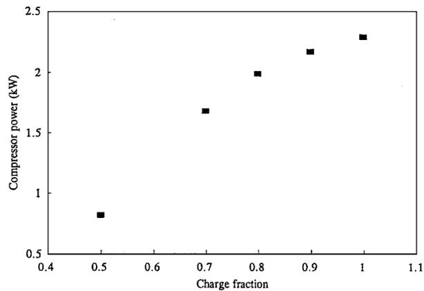
Figure 6. Compressor power versus charge fraction.
