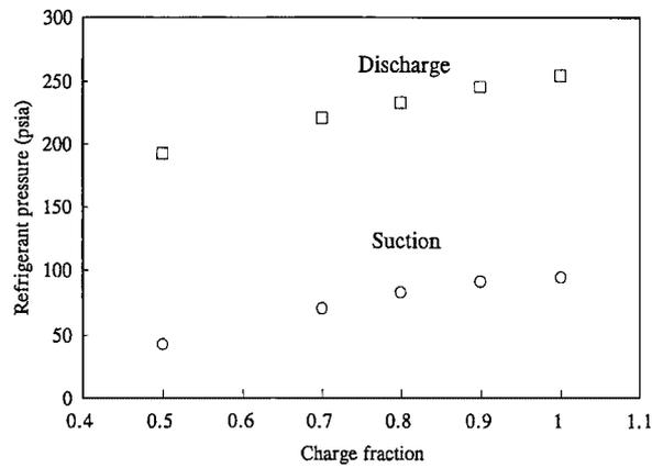
Figure 3. Discharge and suction pressures versus charge fraction.
