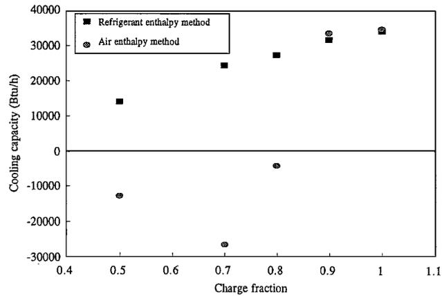
Figure 7. Cooling capacity versus charge fraction.
