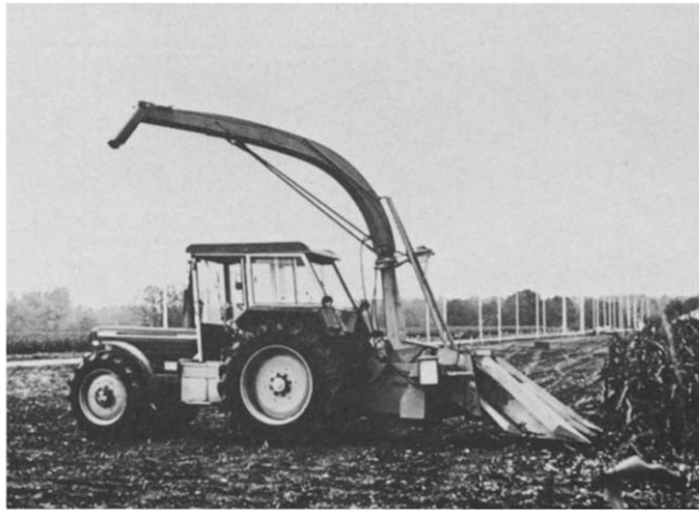
Fig. 12. Tractor and forage harvester operating in the reverse direction
