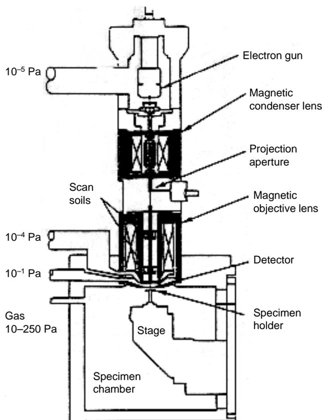
FIG. 2 Environmental scanning electron microscope.
