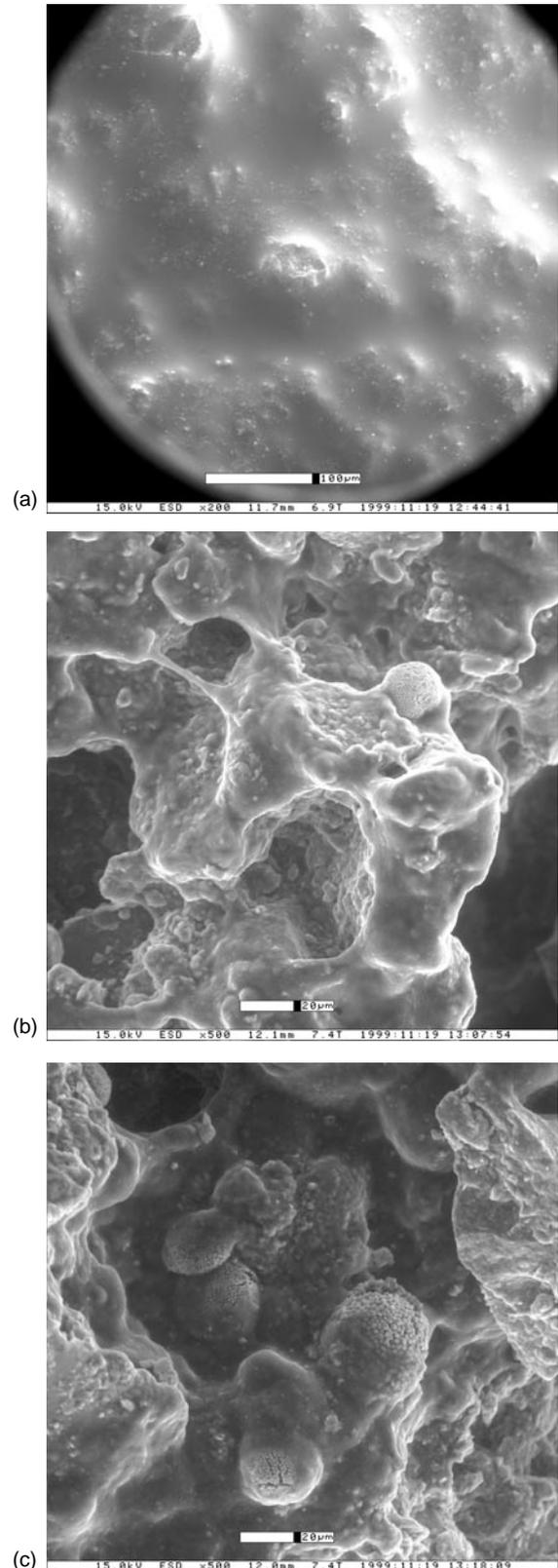
FIG. 4 (a) Environmental scanning electron microscope surface image of the seeded permeability cell (phenol+BOD nutrient) (marker 100  $\mu\text{m}$ ). (b) Bioweb at a greater magnification. (phenol+BOD nutrient) (marker 20  $\mu\text{m}$ ). (c) Bioweb at a greater magnification (phenol+BOD nutrient) (marker 20  $\mu\text{m}$ ).
