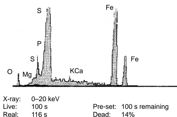
FIG. 5 X-ray microanalysis emission spectra of dehydrated specimen.
