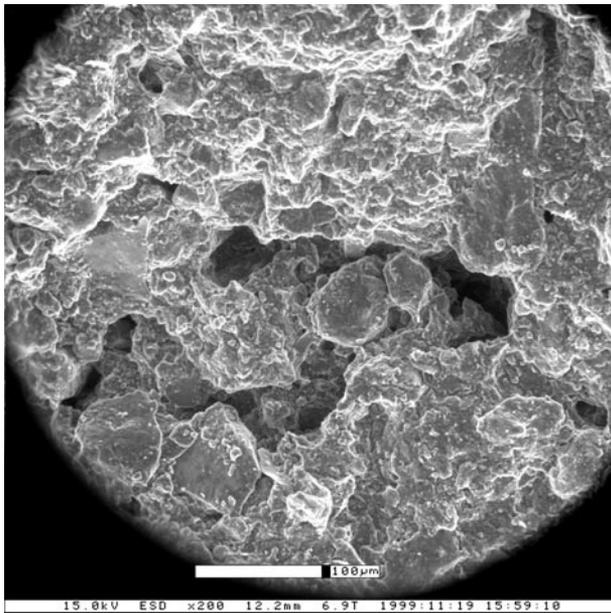
FIG. 3 Environmental scanning electron microscope surface image of the permeability cell containing chemical only (phenol) (marker 100  $\mu\text{m}$ ).
