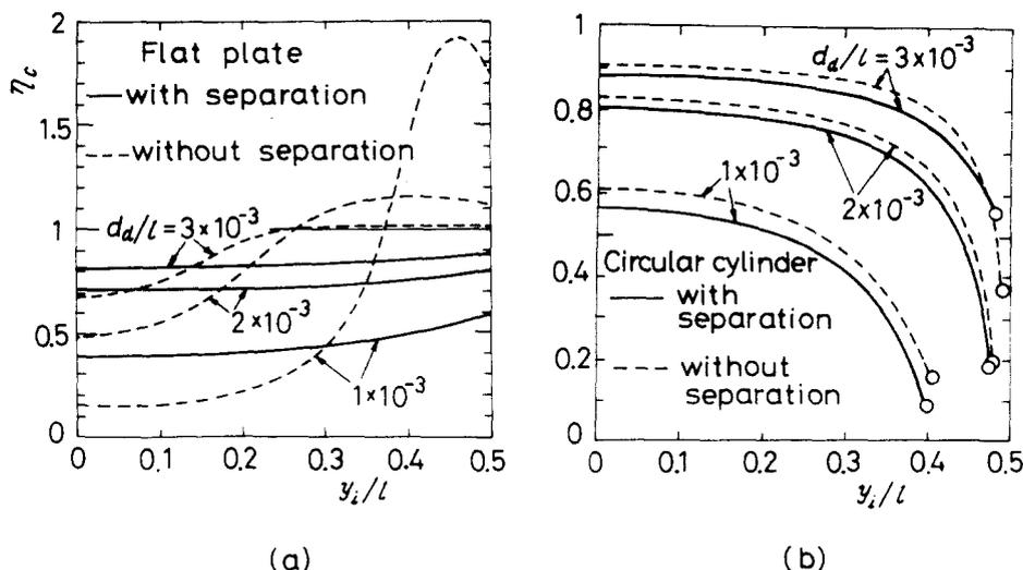
Figure 11. Effect of gas flow separation on local partial collection efficiency  $\eta_c$ .
