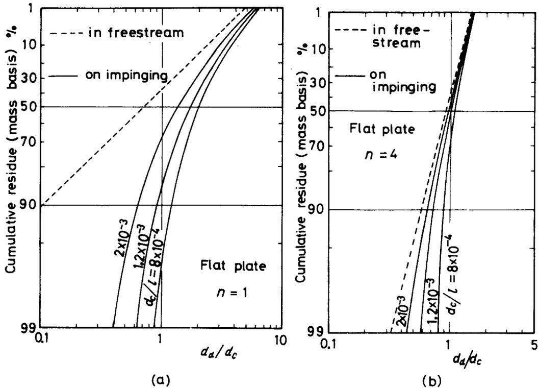
Figure 12. Size distributions of drops in freestream and impinging onto a flat plate.
