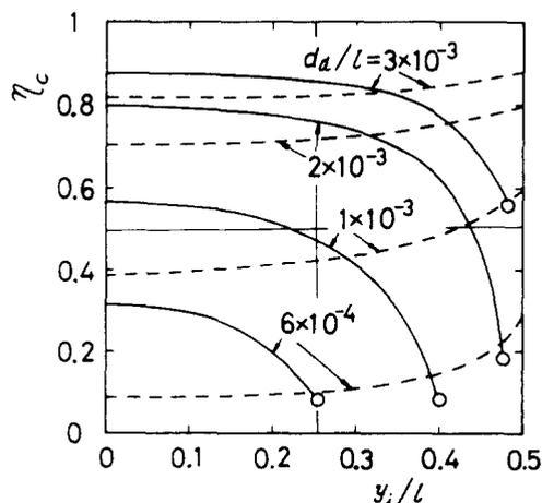
Figure 9. Effect of the droplet diameter  $d_d$  on the distributions of local partial collection efficiency  $\eta_c$ : --- flat plate; — circular cylinder; symbol  $\circ$  refers to the grazing point on the cylinder.
