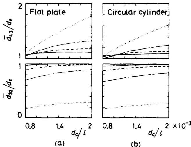
Figure 15. Comparison of the proposed equivalent diameter  $d_e$  with the volume mean diameter  $\bar{d}_{43}$  and surface mean diameter  $\bar{d}_{32}$  in common use.  $\cdots$   $n=1$ ;  $---$   $n=2$ ;  $- \cdot -$   $n=3$ ;  $---$   $n=4$ .
