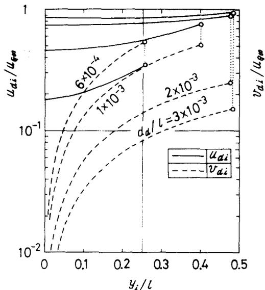
Figure 8. Velocity components  $u_{di}$ ,  $v_{di}$  of droplets impinging onto a circular cylinder. Symbol  $\circ$  refers to the grazing point.
