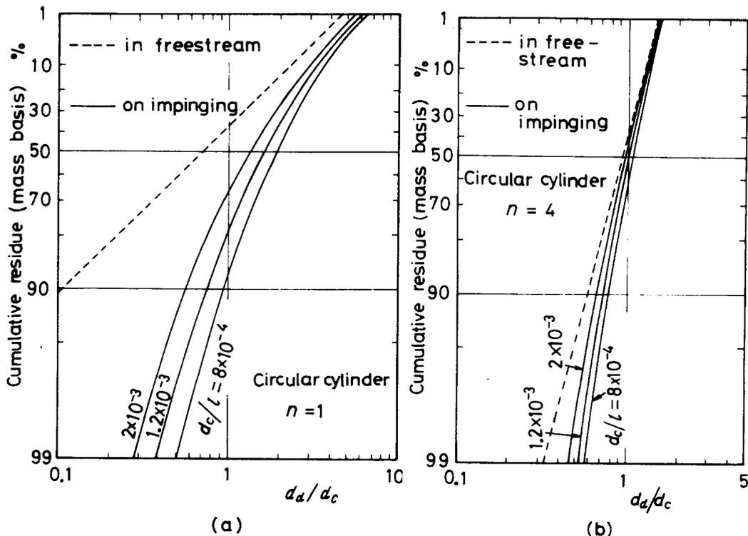
Figure 13. Size distributions of drops in freestream and on impinging onto a circular cylinder.
