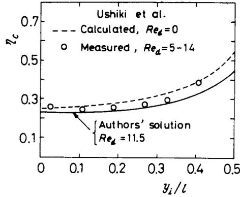
Figure 10. Comparison of the authors' solution with Ushiki *et al.*'s (1977) results in respect of local partial collection efficiency  $\eta_c$  for a normal flat plate ( $K \approx 0.4$ ).
