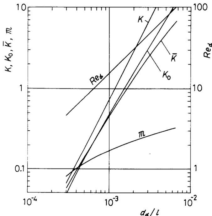
Figure 2. Parameters governing particle trajectories vs  $d_d/l$  ( $Re_G = 1.54 \times 10^4$ ).
