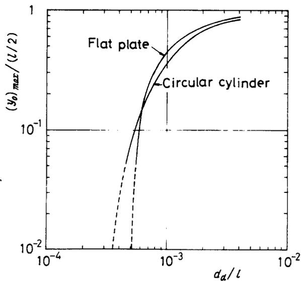
Figure 6. Relations of the starting point  $(y_0)_{max}$  of grazing trajectory to the relative droplet-size  $d_a/l$ : — numerically calculated; --- extrapolated.
