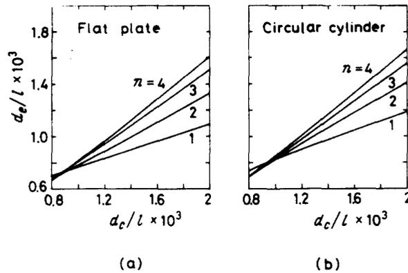
Figure 14. Effect of the droplet size distribution on the proposed equivalent diameter  $d_e$ .
