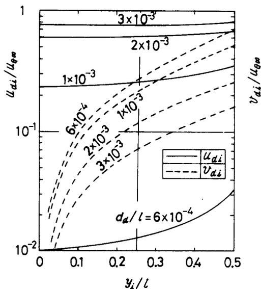
Figure 7. Velocity components  $u_{di}$ ,  $v_{di}$  of droplets impinging onto a normal flat plate.
