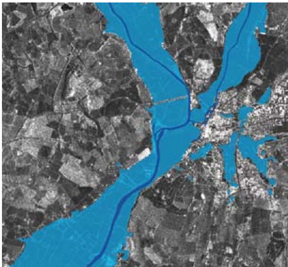
Figure 47 Flood extent around Tewkesbury, England, derived from high-resolution TerraSAR-X data by the use of segmentation-based classification (acquisition date: 25/07/2007; dark blue: normal water level, light blue: flood surface)
