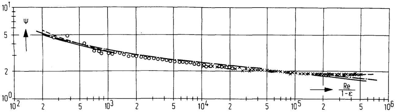
Figure 6. Pressure drop coefficient of pebble beds. (x) High pressure, (o) ambient pressure. — Eq. (21), - - - ref. [22].
