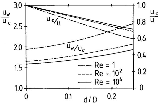
Figure 12. Ratio of wall-to-center and center-to-mean velocities.
