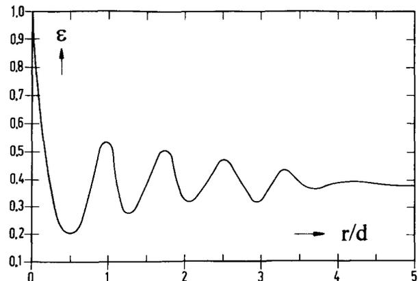
Figure 8. Radial void fraction distribution. (After Ref. 11.)
