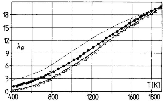
Figure 14. Effective conductivity of packed beds in vacuum and helium. Experiments and theory after Ref. 33; —··· 22.
