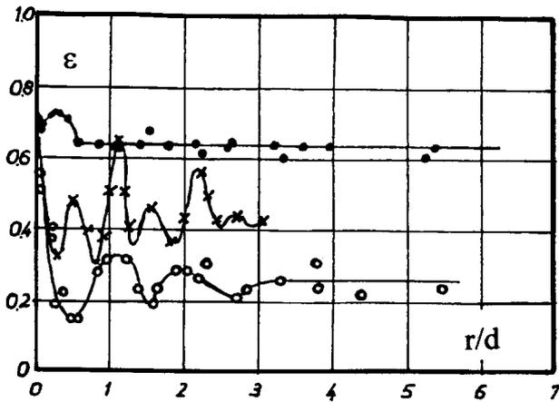
Figure 11. Radial void fraction distribution. Ref. 14: ring (○),  $d_i/d_a = 0.67-0.77$ ; full cylinder (●). Ref. 16: ring (×),  $d_i/d_a = 0.425$ .
