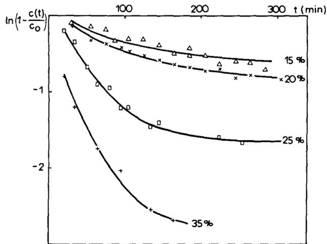
Fig. 11.  $s/l$ -ratio versus time plotted according to the 1st order kinetic of reaction.
