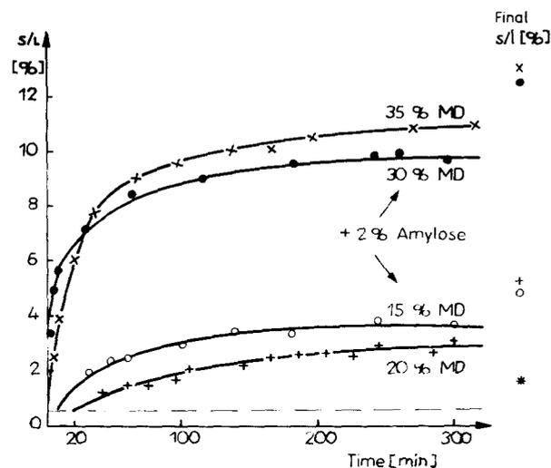
Fig. 6. Action of soluble amylose on the time dependence of the  $s/l$ -values during the initial phase of MD gel forming. (●, ○), solutions with amylose added; (×, and +), pure MD solutions for comparison; (\*), final  $s/l$ -value of the pure amylose solution (% w/w). Half-value times of  $s/l$ : 205 min, 20% MD; 65 min, 15% MD + 2% amylose; 25 min, 35% MD; 10 min, 30% MD + 2% amylose.
