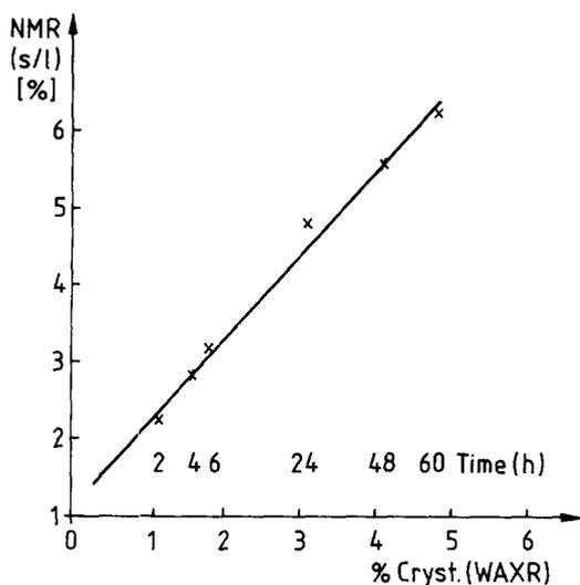
Fig. 10. Linear proportionality between  $s/l$ -values and %-degree of X-ray crystallinity (25% w/w, 20°C).
