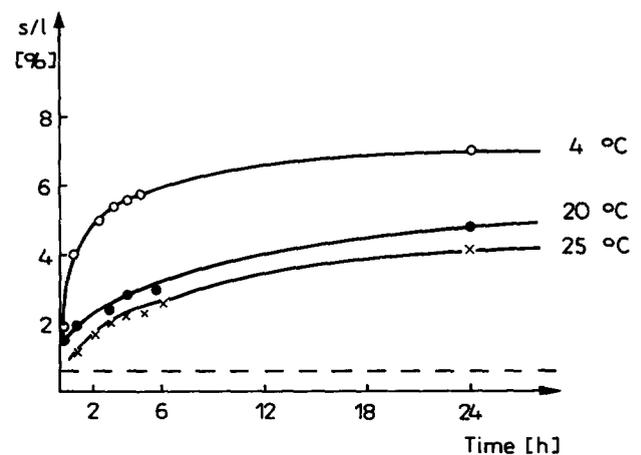
Fig. 4. Time dependence of s/l ratios of 25% (w/w) MD solutions at different temperatures.
