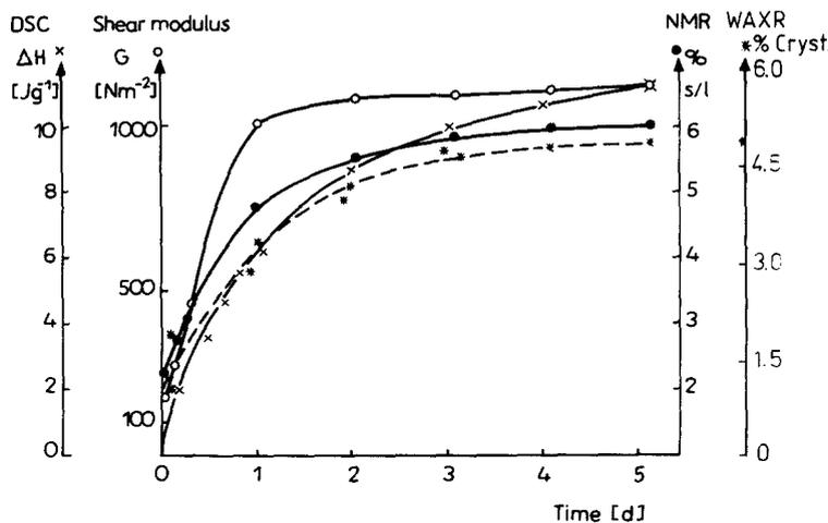
Fig. 9. Time dependence of sol-gel transition of MD-solution as characterized by low resolution-NMR, ●, wide angle X-ray scattering, \*, shear modulus, ○, (20% w/w) and DSC-measurements (8% w/w), ×.
