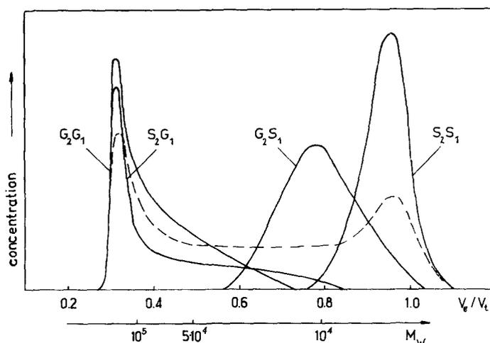
Fig. 2. Gel chromatograms of MD. Triangular fractions:  $G_2G_1$ ,  $\bar{P}_n 250 \pm 40$ ,  $\lambda_{\max} 549$  nm;  $S_2G_1$ ,  $\bar{P}_n 90 \pm 10$ ,  $\lambda_{\max} 552$  nm;  $G_2S_1$ ,  $\bar{P}_n 90 \pm 10$ ,  $\lambda_{\max} 544$  nm;  $S_2S_1$ ,  $\bar{P}_n 10 \pm 2$ ,  $\lambda_{\max} 503$  nm. (---) original maltodextrin (Sephadex G 200, eluant water).
