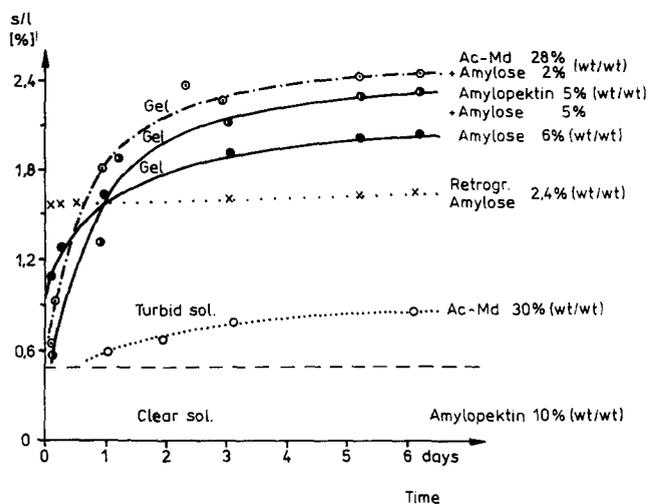
**Fig. 7.** Time dependence of solid-liquid ratio of pure non-gelling solutions of Ac-MD of amylopectin, of amylose solutions and of mixtures thereof.
