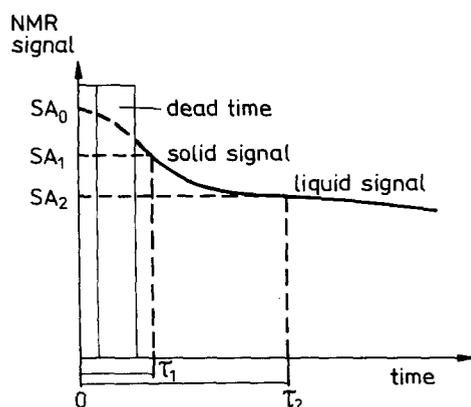
Fig. 1. The free induction decay, which follows the radio frequency radiation pulse worked on for a few microseconds on the probe sample ( $\tau_1$ ,  $\tau_2$ : relaxation times of the entire resp. liquid signal); according to Bruker No. 30 (Bruker, 1988).
