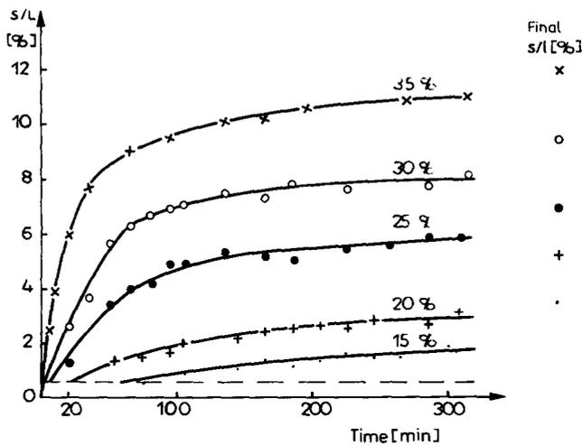
Fig. 3. Time dependence of solid-liquid proton relaxation ratio (s/l) of MD solutions at different concentrations during the first five hours of aggregation (4°C).
