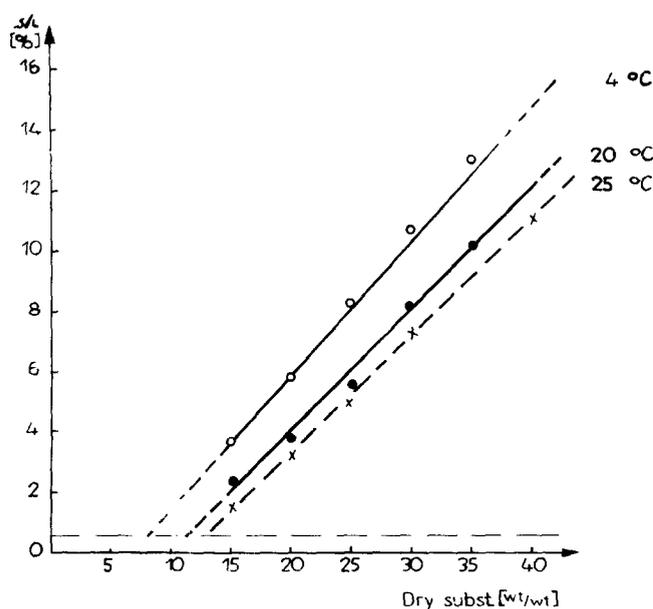
Fig. 5. Dependence of  $s/l$ -values of different MD-solutions on concentration at 4, 20 and 25 °C.
