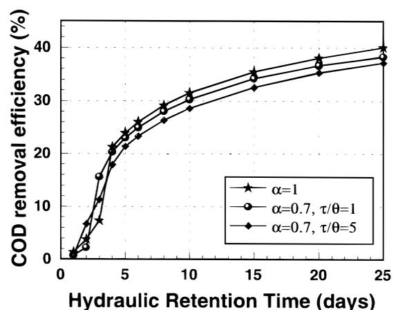
Fig. 6. Effect of the hydraulic retention time on the COD removal efficiency of anaerobic sludge digestion.
