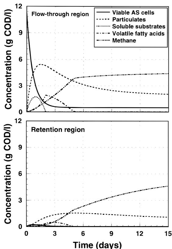
Fig. 4. Dynamic simulation of the anaerobic digestion of waste-activated sludge in a continuous-flow, incompletely mixed reactor ( $\theta = 15$  days;  $\alpha = 0.7$ ;  $\tau = 30$  days).
