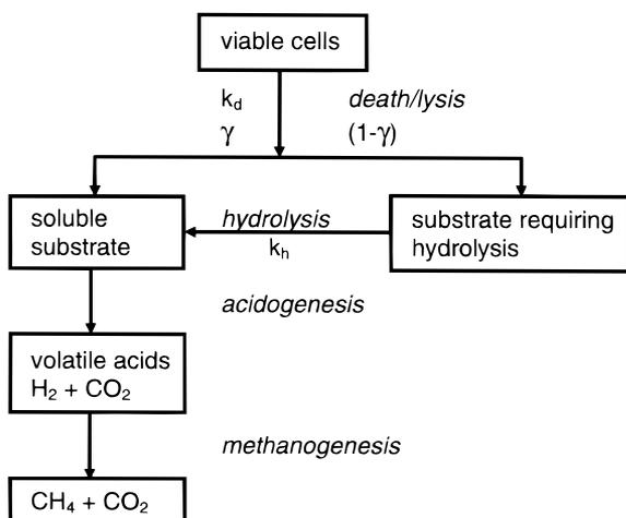
Fig. 1. Conceptual model for the anaerobic digestion of biological sludge (after Pavlostathis and Gossett<sup>9</sup>).
