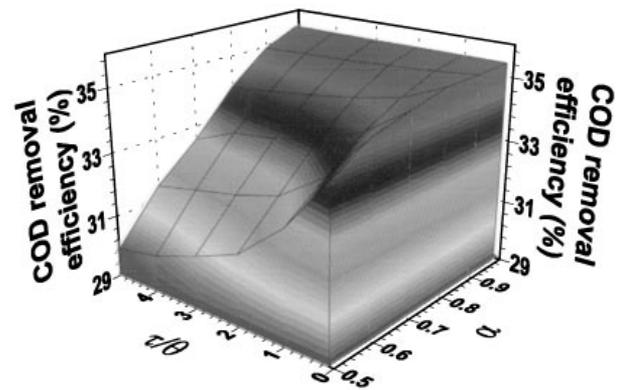
Fig. 9. Effect of the relative volume of the flow-through zone ( $\alpha$ ) and the relative turnover time ( $\tau/\theta$ ) on the COD removal efficiency of anaerobic digestion at steady state conditions ( $\theta = 15$  days).
