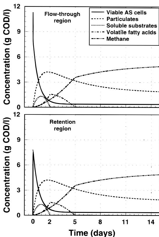
Fig. 5. Dynamic simulation of the anaerobic digestion of waste-activated sludge in a two-regions reactor with non-limited interchange between zones ( $\theta = 15$  days;  $\alpha = 0.7$ ;  $\tau = 0.02$  days).
