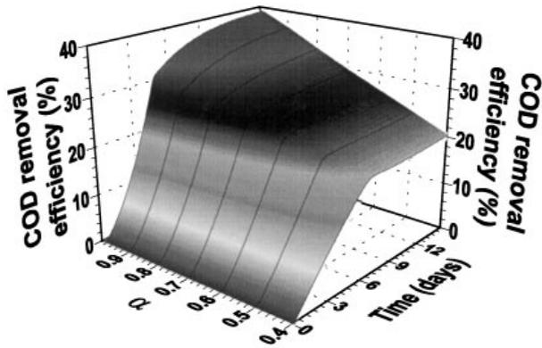
Fig. 7. Effect of the relative volume of the flow-through region ( $\alpha$ ) on the COD removal efficiency of anaerobic sludge digestion under unsteady state conditions ( $\theta = 15$  days,  $\tau/\theta = 2$ ).
