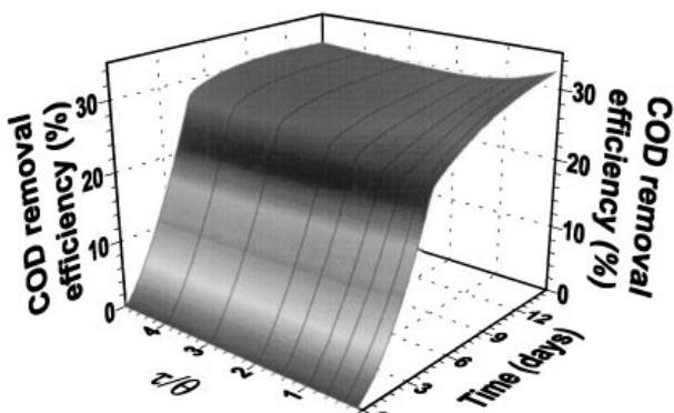
Fig. 8. Effect of the relative turnover time ( $\tau/\theta$ ) on the COD removal efficiency of anaerobic sludge digestion under unsteady state conditions ( $\theta = 15$  days,  $\alpha = 0.7$ ).
