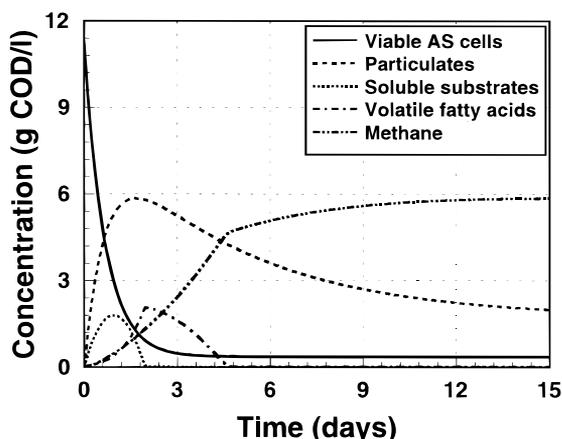
Fig. 3. Dynamic simulation of the anaerobic digestion of waste-activated sludge in a continuous-flow, perfectly mixed reactor ( $\theta = 15$  days).
