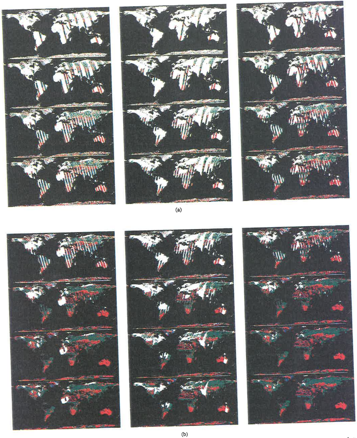
Fig. 9. Swath coverage for the ERS-1 wind-scatterometer over land surfaces (a) from top to bottom: 1, 2, 3, 4 days period and (b) from top to bottom: 5, 10, 20, 30 days period (August 1993).
