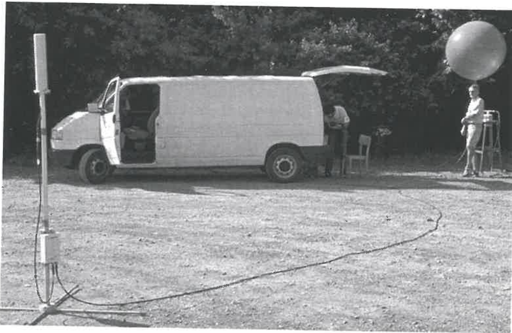
Figure 3.8: The mobile radio sounding unit, in operation during field campaigns (system in courtesy of the Paul Scherrer Institute PSI).
