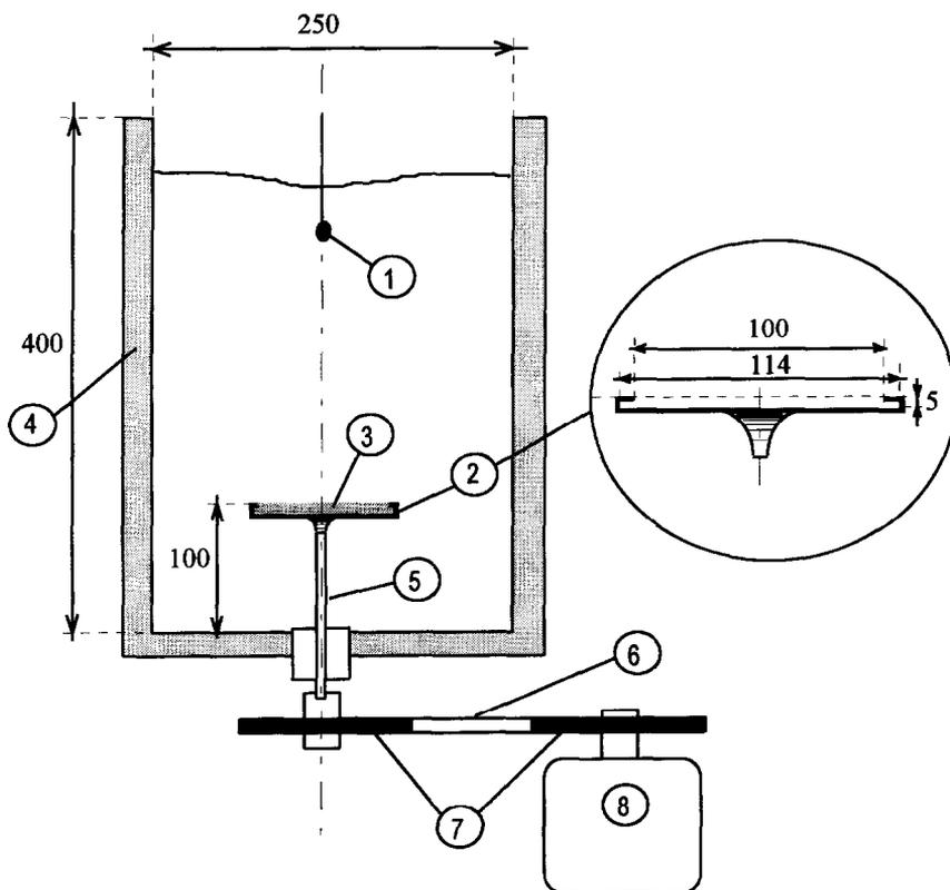
**Fig. 1.** Experimental system: (1) Pt 100 temperature probe; (2) revolving plate; (3) gel disc for processing; (4) freezant fluid; (5) rotation axis; (6) belt; (7) pulley; (8) electric motor.
