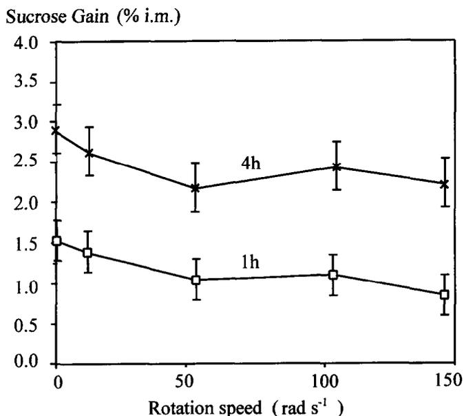
Fig. 4. Influence of rotation speed on sucrose gain in standard gel disc after 1 h (□) and 4 h (×) soaking in ternary liquid ( $m_1 = 6 \text{ mol kg}^{-1}$ ,  $m_2 = 5.55 \text{ mol kg}^{-1}$ ).
