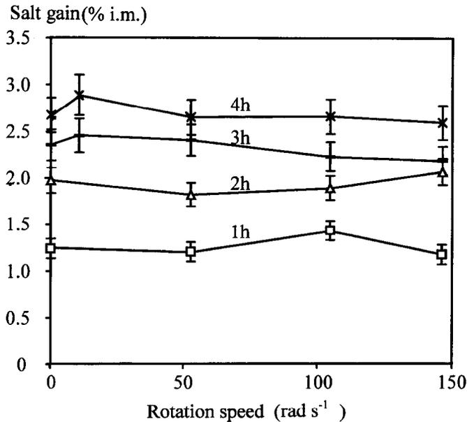
Fig. 3. Influence of rotation speed on salt gain in standard gel disc after 1 h (□), 2 h (△), 3 h (—), and 4 h (×) soaking in ternary liquid ( $m_1 = 6 \text{ mol kg}^{-1}$ ,  $m_2 = 5.55 \text{ mol kg}^{-1}$ ).
