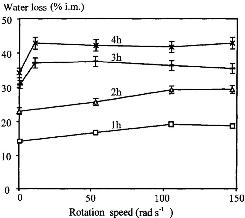
**Fig. 2.** Influence of rotation speed on water loss in standard gel disc after 1 h (□), 2 h (△), 3 h (●), and 4 h (×) soaking in ternary liquid ( $m_1 = 6 \text{ mol kg}^{-1}$ ,  $m_2 = 5.55 \text{ mol kg}^{-1}$ ).
