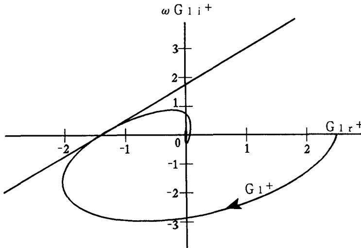
Fig. 5. Modified Nyquist trajectory and Popov straight line for  $G_1(s) = G(s)$ .
