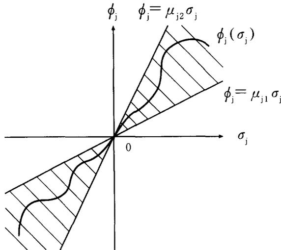
Fig. 1. Sectors enclosing nonlinear function  $\phi(\sigma)$ .
