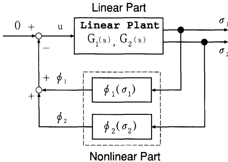
Fig. 3. Fuzzy control system transformed to a Lure's system.
