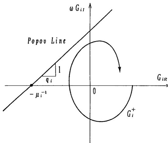
Fig. 4. Modified Nyquist trajectory  $G_i^+$  and Popov straight line.
