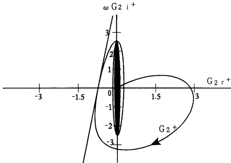
Fig. 6. Modified Nyquist trajectory and Popov straight line for  $G_2(s) = sG_1(s)$ .
