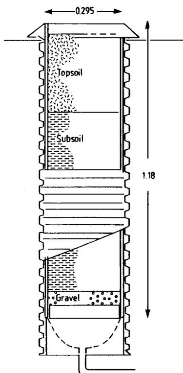
Fig. 1. Lysimeter placed in a below-ground pipe (from Bergström & Johansson, 1991).
