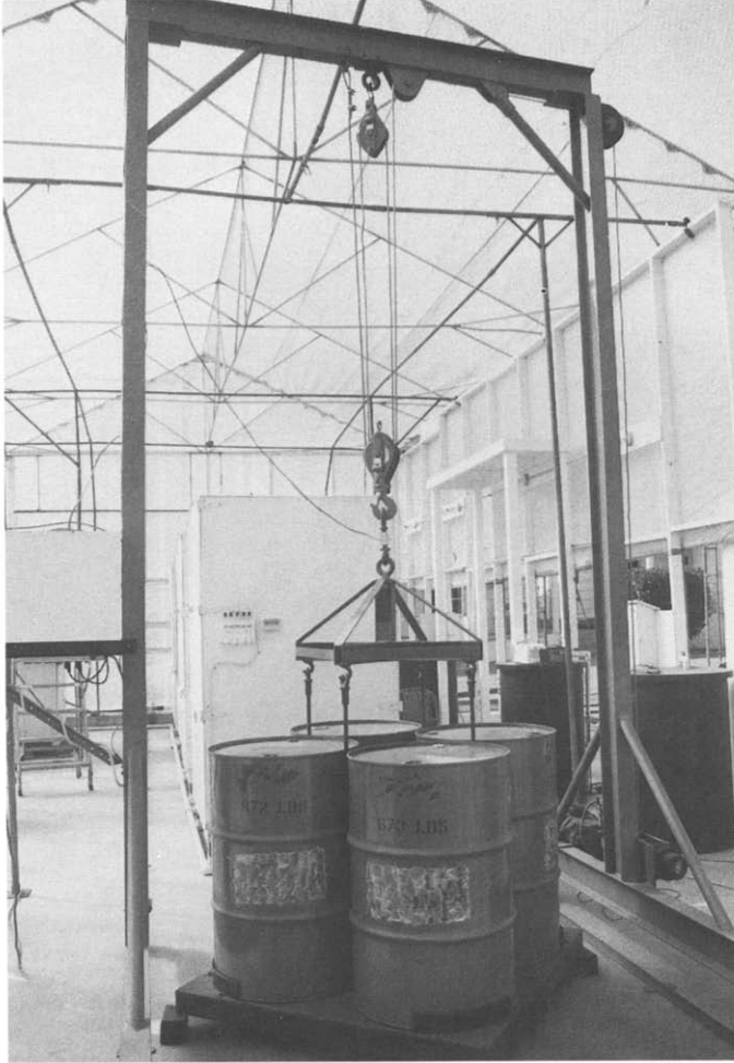
Fig. 8. Hoist, load cell and calibration weights of the soil lysimeter weighing apparatus.
