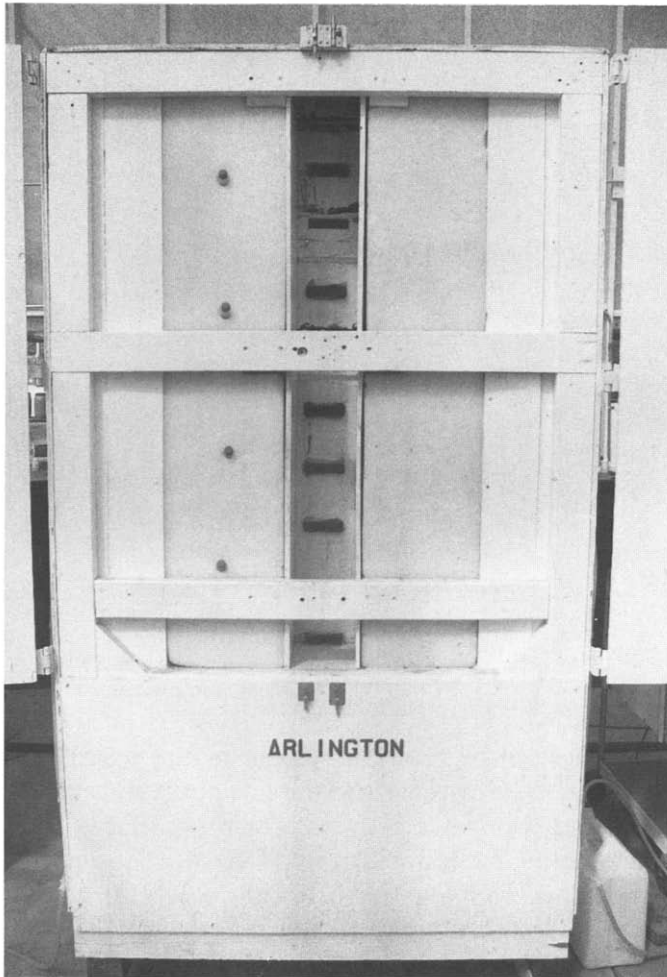
Fig. 7. Instrument placement of TDR rods and tensiometers along one side of a lysimeter.
