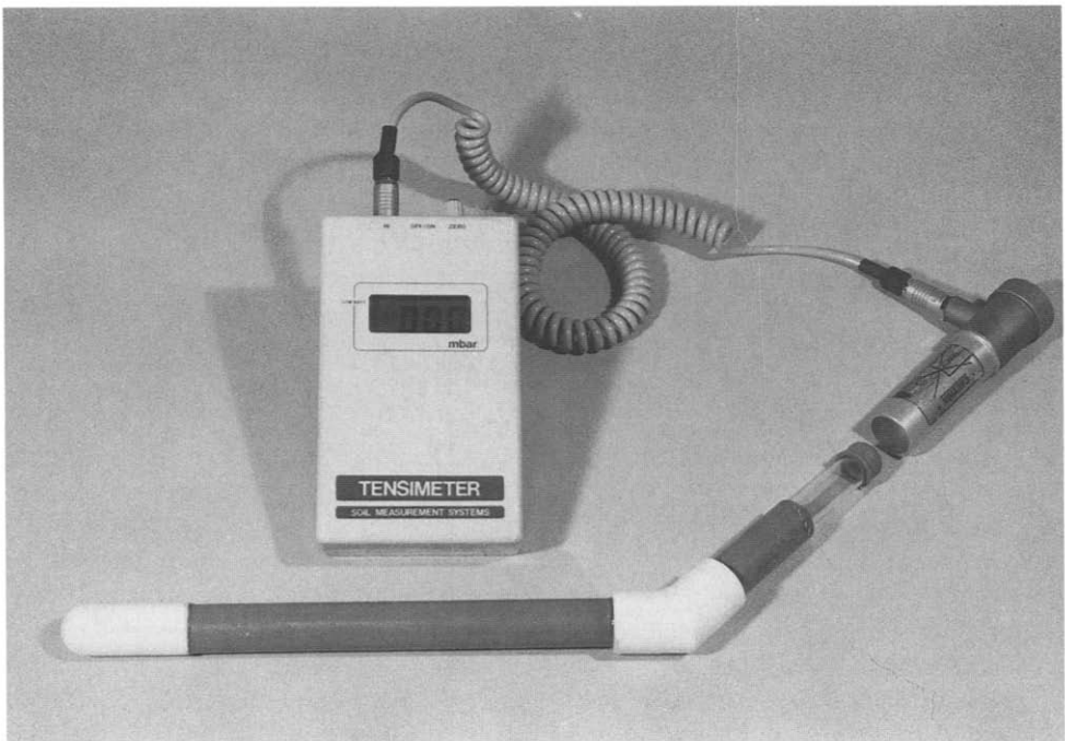
Fig. 5. Photograph showing a soil tensiometer and the Tensimeter ® recorder which is used to read matric potential quickly and easily.
