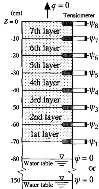
Fig. 3. Schematic of simulated soil profile with location of tensiometers and imposed boundary conditions, showing the numbering system of soil layers and capillary pressures. The hydraulic properties of soil below the 1st layer are the same as those of the uniform soil column (material A in Table 1).
