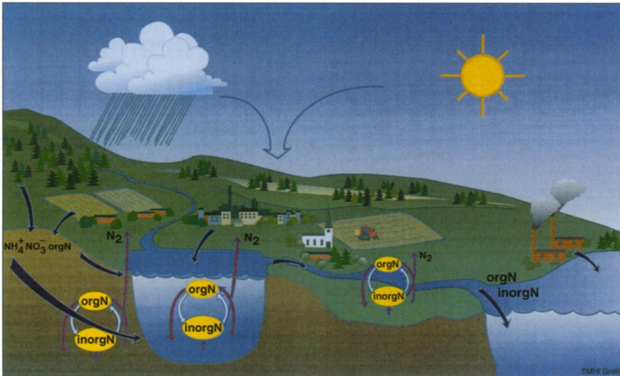
**Figure 2.** Illustration of the system modelled by the HBV-N model. The nitrogen transport simulations are based on the water discharge received by the hydrological HBV model, mixing of water with different concentrations, and simple functions describing the net influence from various biogeochemical processes affecting the nitrogen load during the residence time in discharge areas, rivers and lakes.
