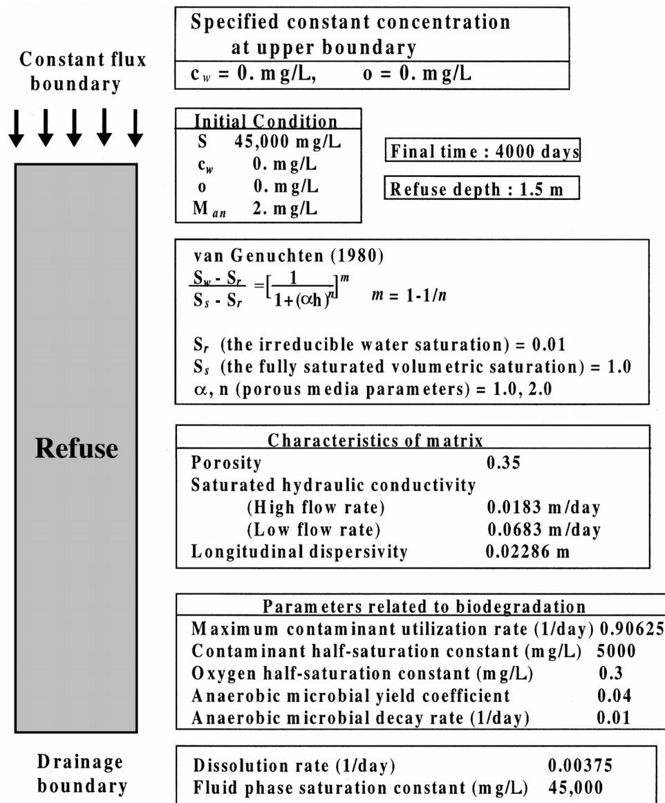
FIG. 5. Input Parameters and Conceptual Model for Application
