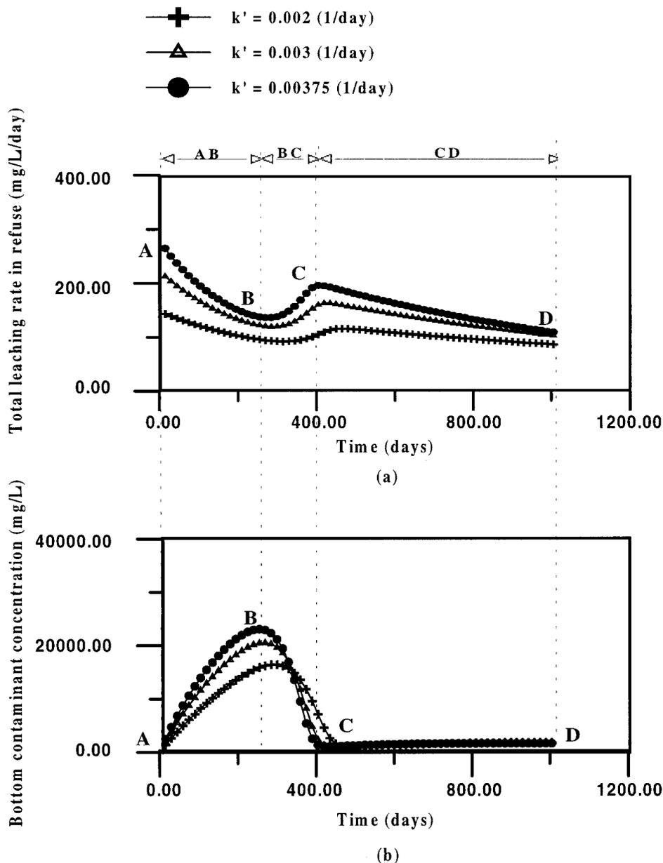
**FIG. 4.** Sensitivity Analysis of: (a) Total Leaching Rate in Refuse; (b) Bottom Contaminant Concentration; (c) Bottom Biomass Concentration; (d) Total Remaining Solid Waste Fraction in Refuse to Dissolution Rate
