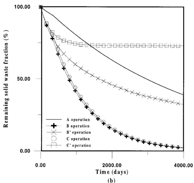
**FIG. 6.** History of: (a) Simulated Bottom Leachate Concentrations; (b) Simulated Total Remaining Leachable Solid Waste Fractions with Time for Leachate Recirculation and Continued Input of Pure Water with Relatively Low Flow Rate ( $5.26E-4$  m/day) and Landfill Control with Leakage Rate ( $2.13E-6$  m/day), Considering Microbial and No Microbial Activity
