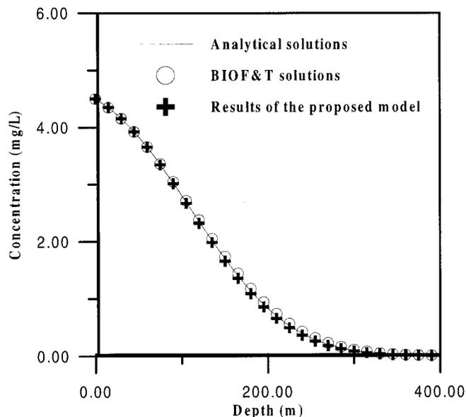
**FIG. 1.** Comparison of Solutions of Proposed Model with Analytical and BIOF&T Solutions in Nonreactive Transport Problem at 6,000 days (Specified Constant Concentration at Inflow Boundary = 4.5 mg/L)
