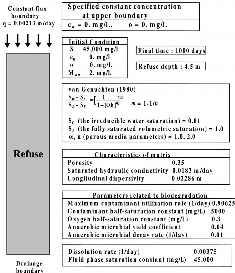
FIG. 3. Input Parameters and Conditions for Sensitivity Analysis
