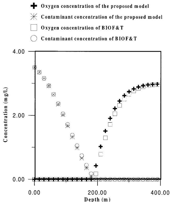
**FIG. 2.** Comparison of Solutions of Proposed Model with BIOF&T Solutions in Biologically Reactive Transport Problem at 6,000 Days (Specified Constant Concentrations of Contaminant and Dissolved Oxygen at Inflow Boundary = 4.5 and 3 mg/L, Respectively)
