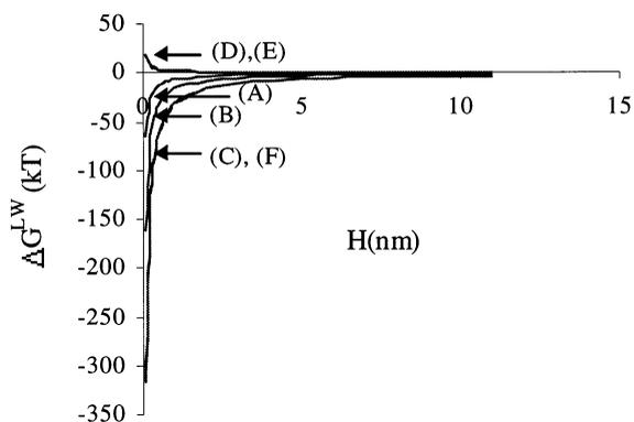
Fig. 3. Variation of the free energy of the van der Waals interaction between the mutants TR (A), CV (B) and F72 (C) and glass when immersed in PBS and between the mutants TR (D), CV (E) and F72 (F) and glass when immersed in EPS as a function of the distance of separation ( $H$ ).
