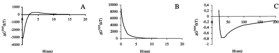
Fig. 8. Variation of the XDLVO total free energy of interaction between the mutants TR (A), CV (B) and F72 (C) and glass when immersed in EPS as a function of the distance of separation ( $H$ ).
