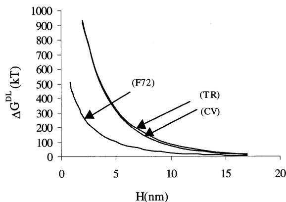
Fig. 2. Variation of the free energy of the electrostatic interactions ( $\Delta G^{DL}$ ) between the mutants TR, CV and F72 and glass immersed in EPS as a function of the distance of separation ( $H$ ).
