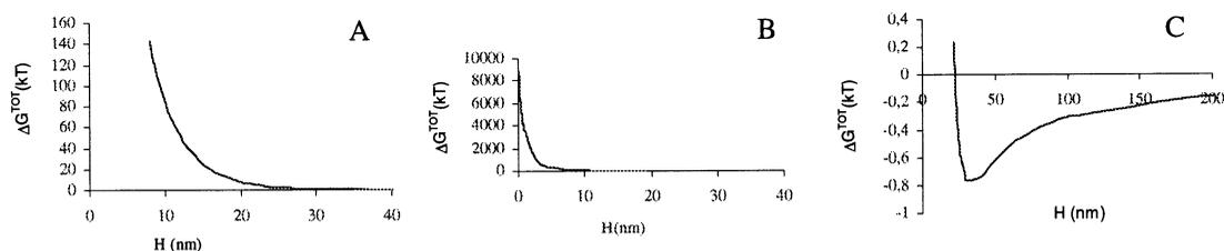
Fig. 5. Variation of the total DLVO free energy of interaction between the mutants TR (A), CV (B) e F72 (C) and the glass when immersed in EPS as a function of the distance of separation ( $H$ ).
