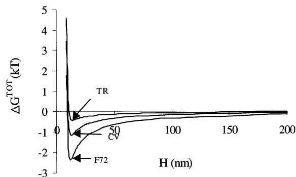
Fig. 7. Variation of the XDLVO total free energy of interaction between the mutants TR, CV e F72 and glass when immersed in PBS as a function of the distance of separation ( $H$ ).
