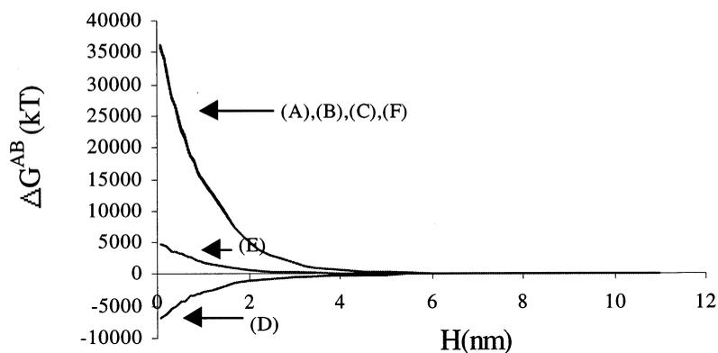
Fig. 6. Variation of the polar free energy of interaction between the mutants TR (A), CV (B) and F72 (C) and glass when immersed in PBS and between the mutants TR (D), CV (E) and F72 (F) and glass when immersed in EPS as a function of the distance of separation ( $H$ ).
