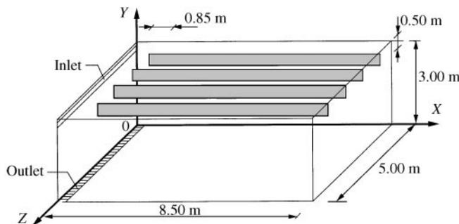
Fig. 6. The experimental room with ceiling guiding plates installed
