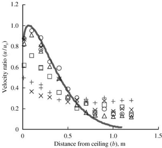
Fig. 3. Velocity profiles of the ceiling jet in five  $z$ -planes at the horizontal distance  $x$  of 4.5 m from the inlet wall:  $\times$ ,  $z$  of 0.5 m;  $\square$ ,  $z$  of 1.5 m;  $\circ$ ,  $z$  of 2.5 m;  $\triangle$ ,  $z$  of 3.5 m;  $+$ ,  $z$  of 4.5 m; —, Eqn (2);  $u$ , air velocity in jet;  $u_x$ , maximum air velocity in jet at distance  $x$  from inlet;  $b$ , vertical distance from ceiling
