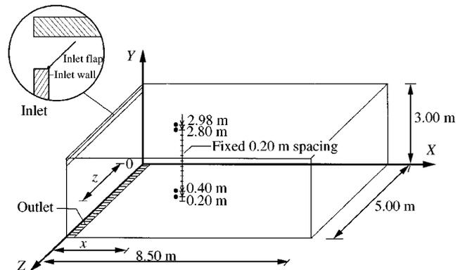
*Fig. 1. Room geometry and positions of inlet, outlet and sensors. The horizontal distances  $x$  from the sensors to the inlet wall were 2.68, 3.50 and 4.50 m, and the horizontal distance  $z$  from the side-wall were 0.5, 1.5, 2.5, 3.5 and 4.5 m*
