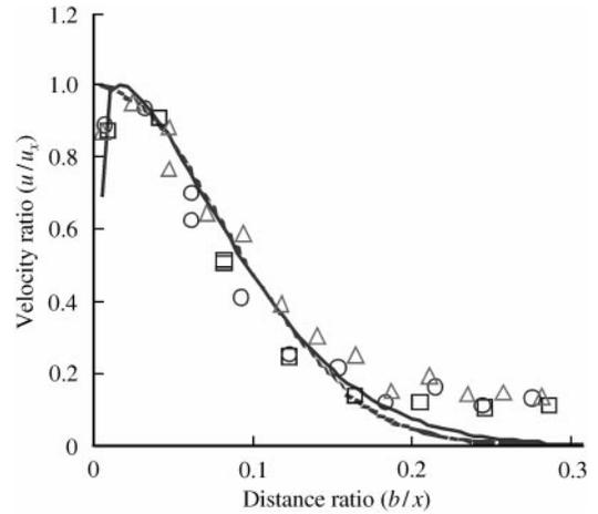
Fig. 2. Velocity profiles of the ceiling jet in the symmetrical plane at  $z$  of 2.5 m for the different values of the horizontal distance  $x$  downstream from the inlet:  $\square$ ,  $x$  of 2.68 m;  $\circ$ ,  $x$  of 3.5 m;  $\triangle$ ,  $x$  of 4.5 m; —, Eqn (2); ---, Eqn (4);  $u$ , air velocity in jet;  $u_x$ , maximum air velocity in jet at distance  $x$  from inlet;  $b$ , vertical distance from ceiling
