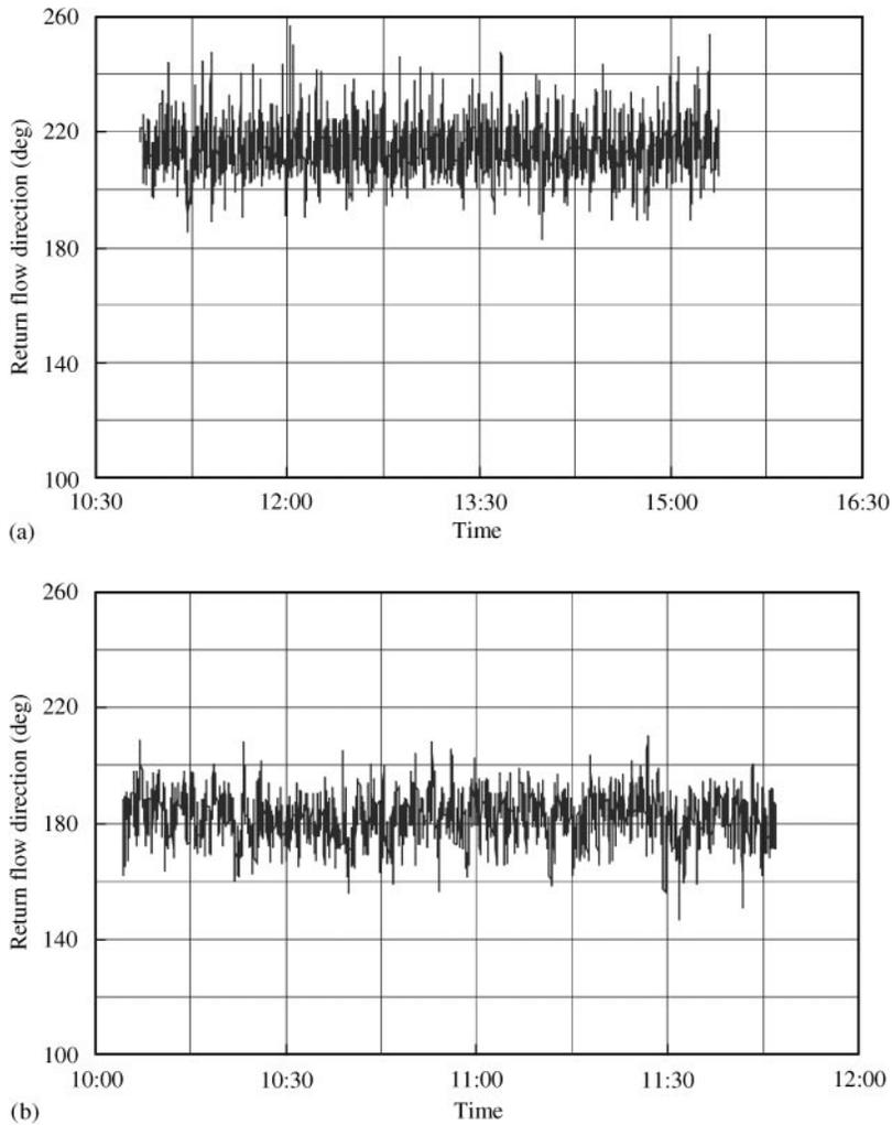
Fig. 5. Return airflow direction measured at  $x$  of 6.5 m,  $y$  of 0.2 m and  $z$  of 2.5 m, with and without ceiling guiding plates: (a) without ceiling guiding plates; (b) with ceiling guiding plates
