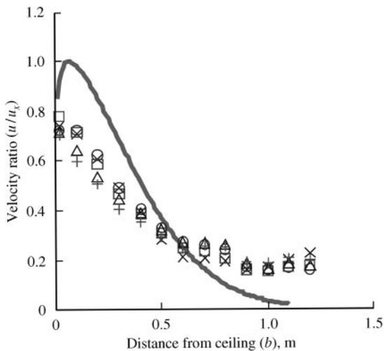
Fig. 7. Velocity profiles of the plane, attached jet at a distance  $x$  of 4.5 m downstream from the inlet wall in the room with guiding plates:  $\times$ ,  $z$  of 0.5 m;  $\square$ ,  $z$  of 1.5 m;  $\circ$ ,  $z$  of 2.5 m,  $\triangle$ ,  $z$  of 3.5 m,  $+$ ,  $z$  of 4.5 m; —, Eqn (2). air velocity in jet;  $u_x$ , maximum air velocity in jet at distance  $x$  from inlet;  $b$ , vertical distance from ceiling
