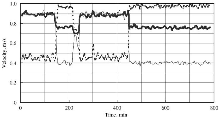
Fig. 4. Velocities measured in the ceiling jet at the distance  $x$  of 4.5 m from the inlet wall, a distance of 0.2 m from ceiling and at three distances  $z$  from the side-wall: ---,  $z$  of 0.5 m; —,  $z$  of 2.5 m; —,  $z$  of 4.5 m. The semi-stable airflow state in the room is clearly illustrated
