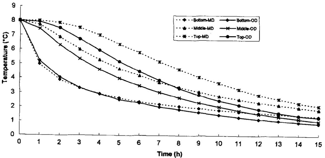
Fig. 11. Cooling curves for beetroot at top, middle and bottom of bins in wet air-cooled store (OD = original design, MD = air circulation rate decreased by 20%).
