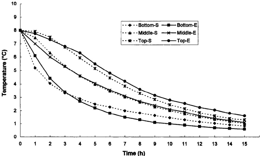
Fig. 4. Cooling curves of beetroot at top, middle and bottom of the bins in the wet air-cooled store (E = experiment, S = simulation).
