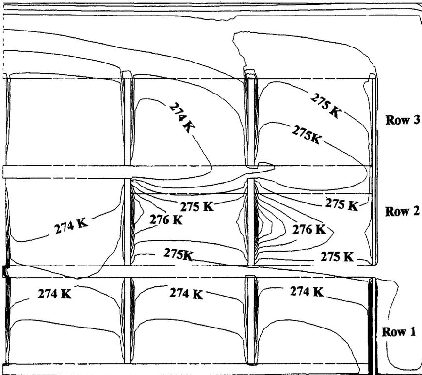
**Fig. 9.** Average produce temperature distribution in the modified cold store after 15 h operation (the height of the produce in the middle and right bins of the middle row has been changed).
