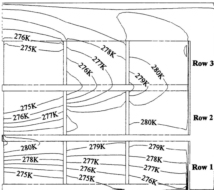
Fig. 6. Average produce temperature distribution in the wet air-cooled store after 5 h operation.
