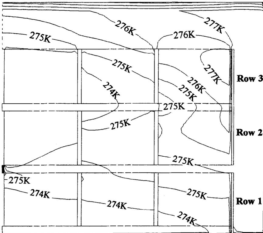
Fig. 8. Average produce temperature distribution in the wet air-cooled store after 15 h operation.
