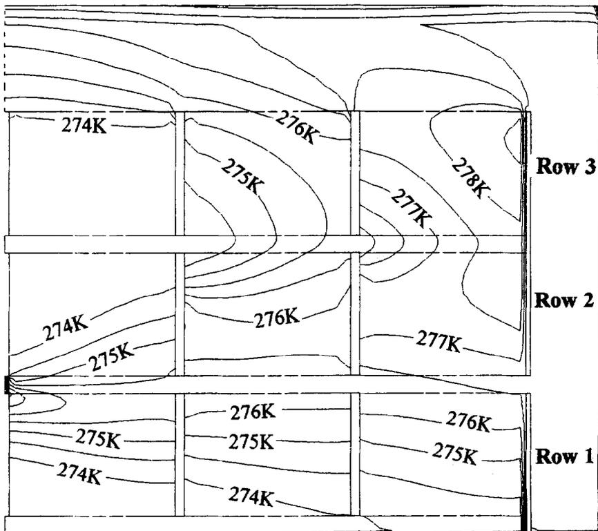
Fig. 7. Average produce temperature distribution in the wet air-cooled store after 10 h operation.
