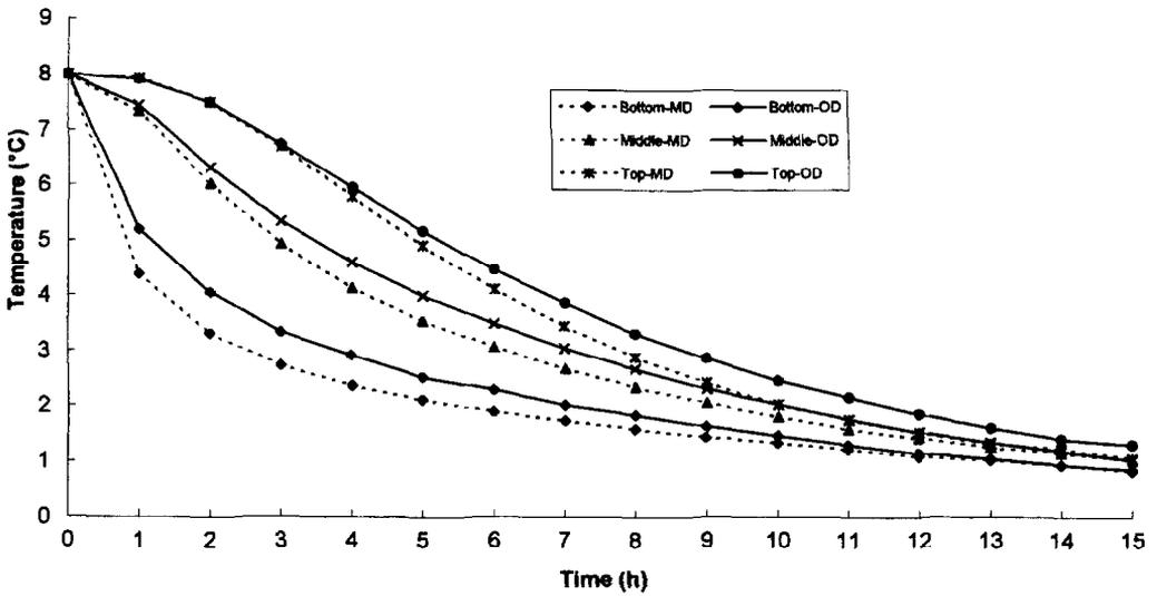
Fig. 10. Cooling curves for beetroot at top, middle and bottom of bins in wet air-cooled store (OD = original design, MD = air circulation rate increased by 20%).
