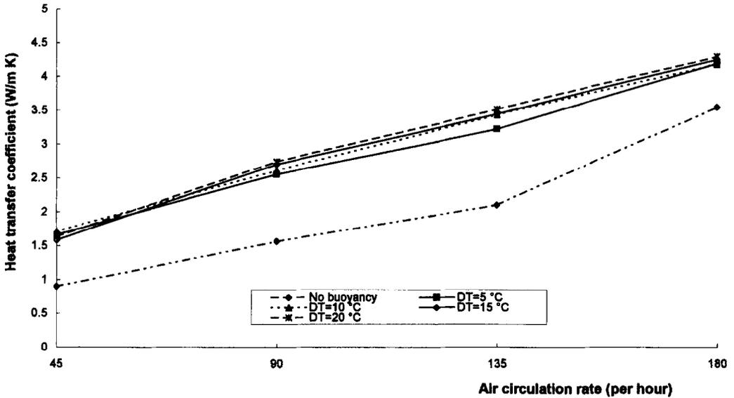
Fig. 3. Effect of buoyancy on the overall heat transfer coefficient in cold store.
