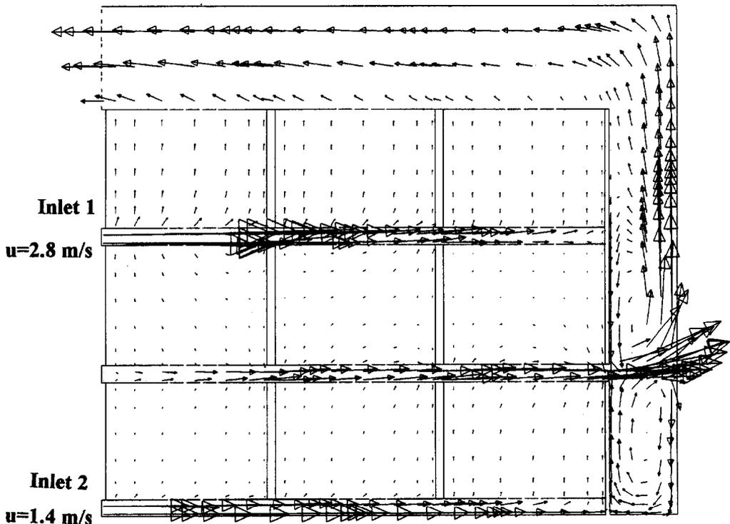
Fig. 5. Velocity distribution in the wet air-cooled store.
