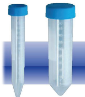
Figure 1. Falcon tubes (15 ml and 50 ml), ideal for centrifuging concentrated plankton samples and subsequent processing to extract toxins. They can also be used to hold the folded filter.
