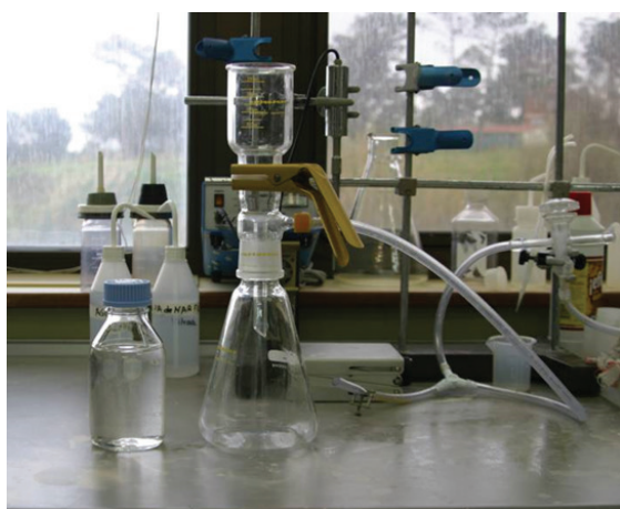
Figure 2. Filtration equipment (filter holder) with a vacuum pump connected to the water tap in the sink. Right: colour of plankton accumulated in the glass-fibre filter (Photo: P. Riobó).
