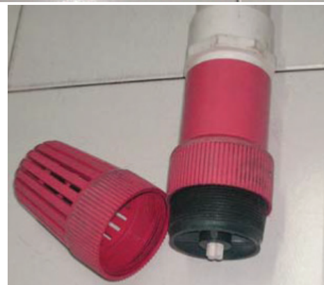
Figure 9. Close-up of a check valve used with a tube measuring two inches in diameter (Photo: INVEMAR, Colombia).
