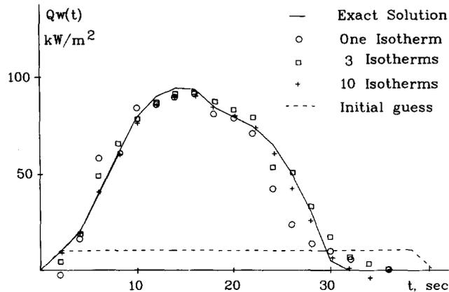
Figure 4 The heat flux estimation using 1, 3, and 10 isotherms with precise data
