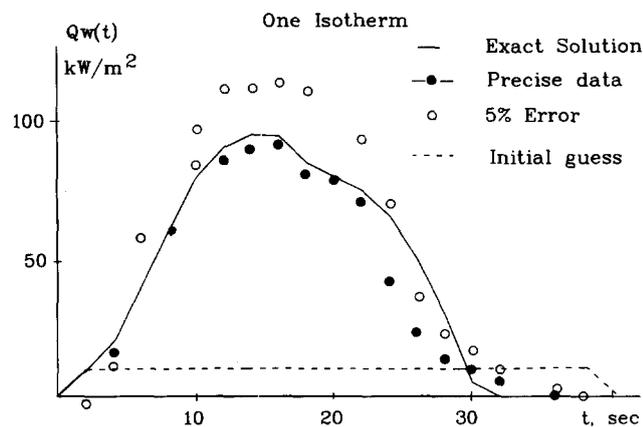
Figure 5 The heat flux estimation using one isotherm for 0 and 5% standard deviation error in input data
