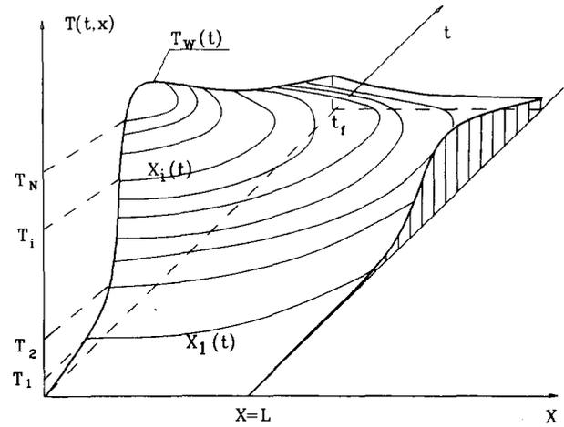
Figure 2 The temperature field and coordinate of color change in time dependence
