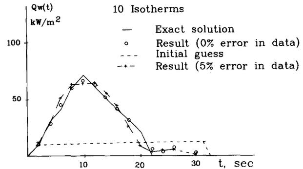
Figure 6 The heat flux estimation using 10 isotherms for 0 and 5% standard deviation error in input data
