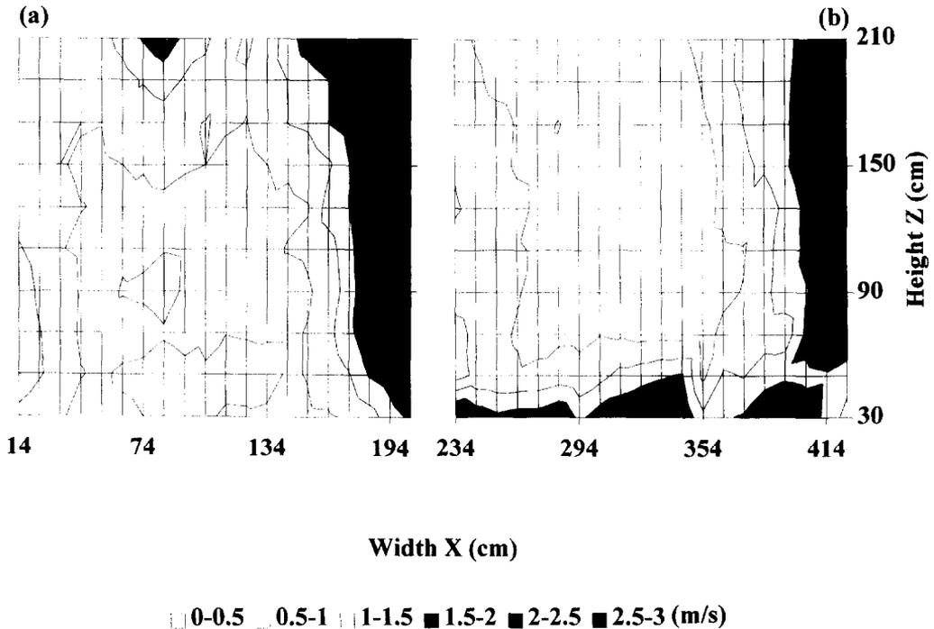
Fig. 9. Distribution of the measured air velocities in the small-scale chiller in a vertical section located at a length  $Y$  of 405 cm (a) in the blowing part (b) in the suction part.
