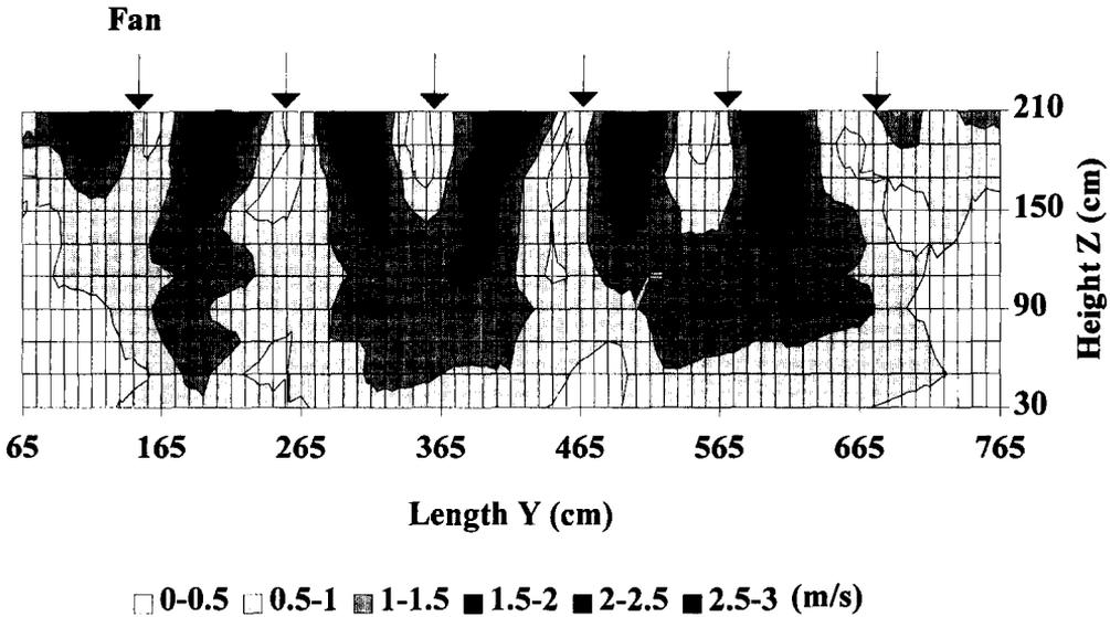
Fig. 8. Distribution of the measured air velocities in the small-scale chiller in a longitudinal section located at a width  $X$  of 174 cm, i.e. in the axis of the second fan row.
