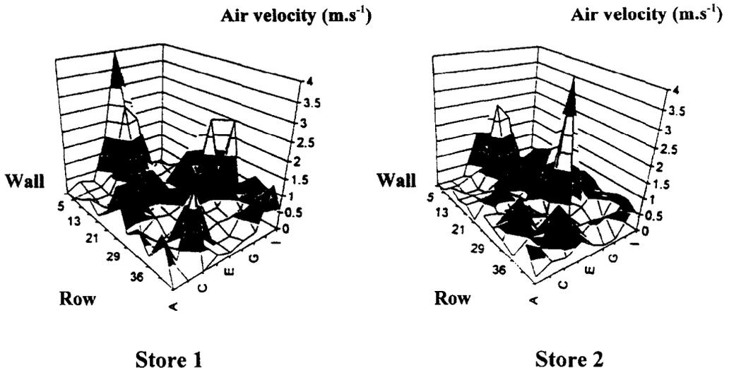
**Fig. 1.** Graphical representation of the mean air velocities measured in a horizontal section in two cheese stores of similar dimensions, but with different air flow rates:  $136\,000\text{ m}^3\text{ h}^{-1}$  in the case of store 1 and  $102\,000\text{ m}^3\text{ h}^{-1}$  in the case of store 2 (from Falconer, 1993).
