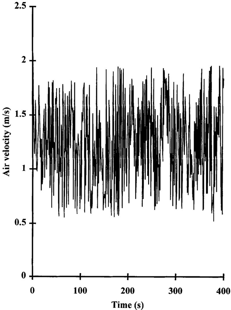
**Fig. 2.** Variations in the air velocity magnitude due to flow unsteadiness and turbulence at one fixed location in an industrial meat chiller (air velocities were recorded using a hot-film type anemometer and an acquisition frequency of 1 Hz).
