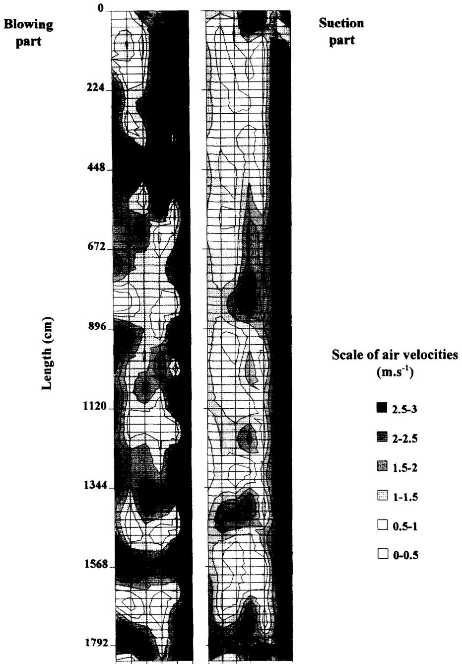
**Fig. 11.** Distribution of the air velocities in an industrial pork offal chiller in a horizontal section located at 70 cm above the ground (the velocities were calculated after processing the measurements carried out in our laboratory, with the new experimental method).
