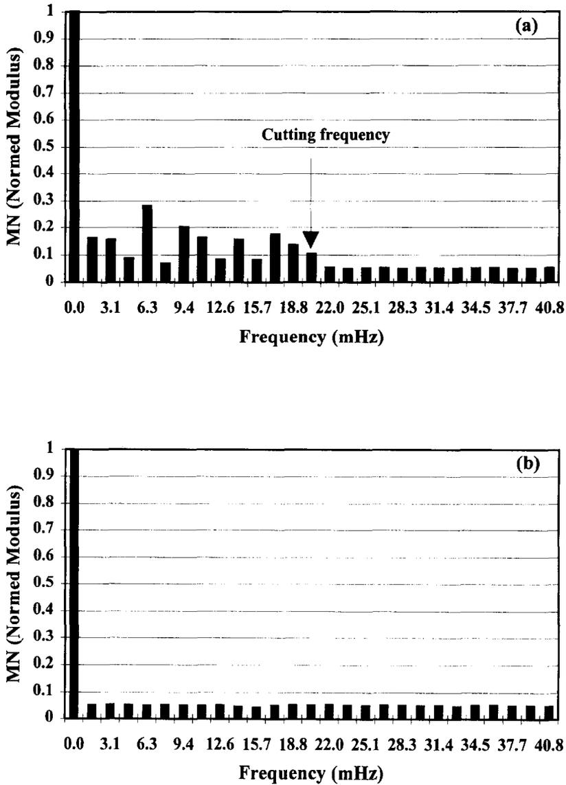
**Fig. 3.** Graphical representation of the mean spectra representing the air velocity measurements performed (a) by moving and (b) without moving the hot-film type anemometer in a small-scale chiller (the mean spectrum shown in Fig. 3(b) was obtained at one fixed location and it was really representative of what could be performed anywhere in the room).
