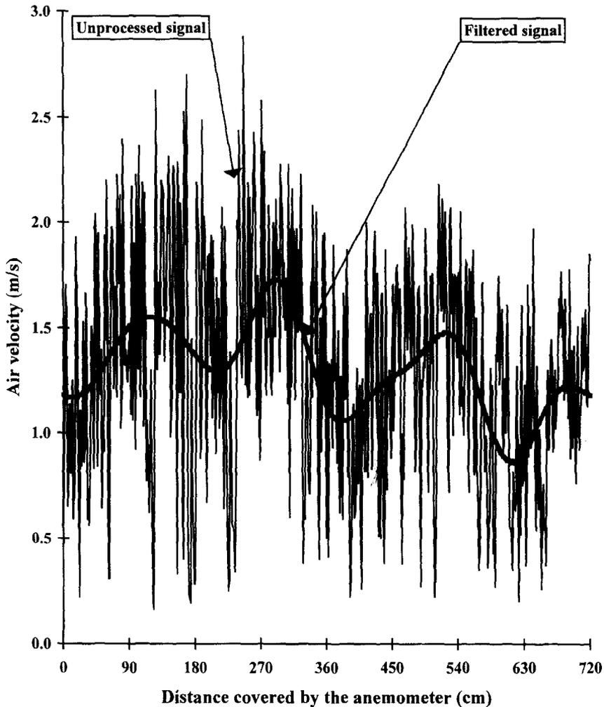
**Fig. 4.** Example of a filtered signal at 20 mHz corresponding to air velocity measurements carried out in the small-scale chiller by moving the hot-film type anemometer at a velocity of  $1.2 \text{ cm s}^{-1}$  and using an acquisition frequency of 1 Hz.
