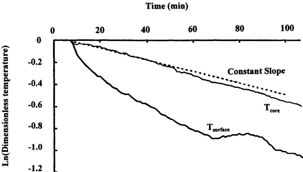
Fig. 10. Variation of the logarithm of the dimensionless temperatures measured in a pork liver of 1.5 kg moving in an industrial chiller (from Daudin *et al.*, 1992).
