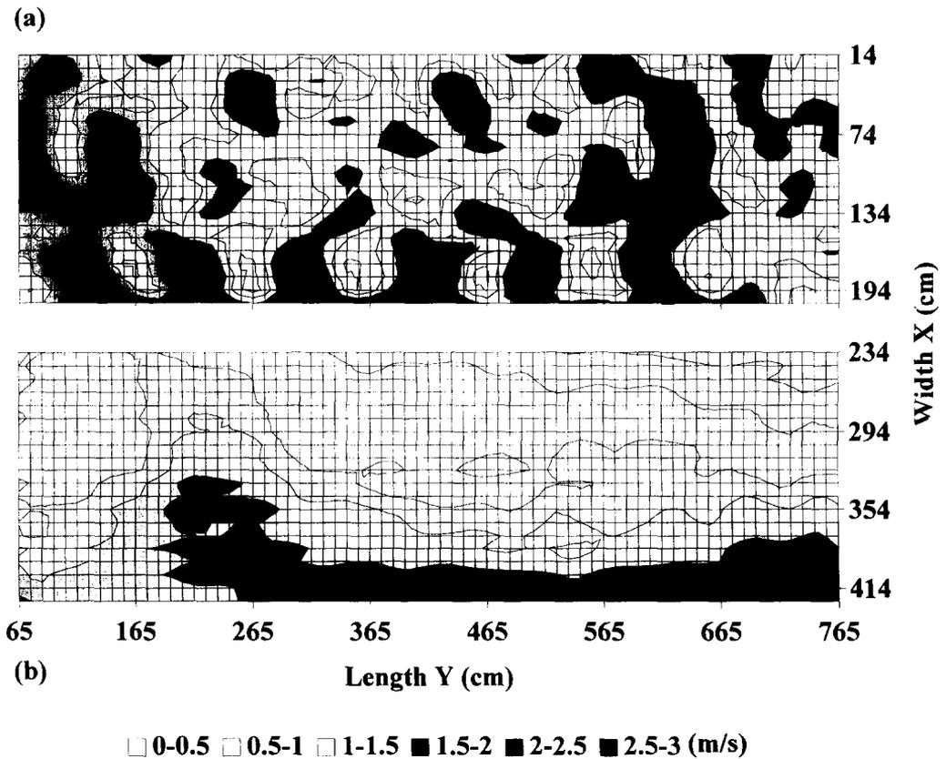
Fig. 7. Distribution of the measured air velocities in the small-scale chiller in a horizontal section located (a) in the blowing part at 90 cm below the blowing of fans and (b) in the suction part at 2.1 m above the ground.
