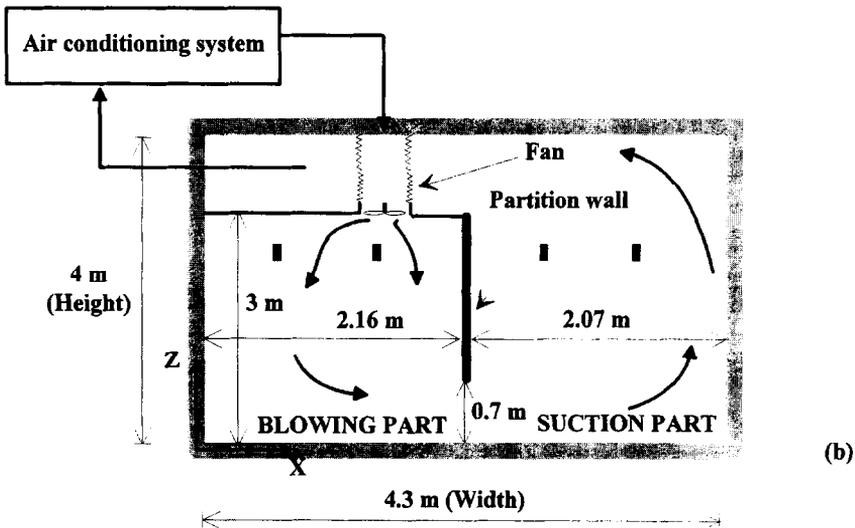
Fig. 6. Description of the geometry of the small-scale chiller: (a) top view (b) vertical section with a schematic description of the air flow.
