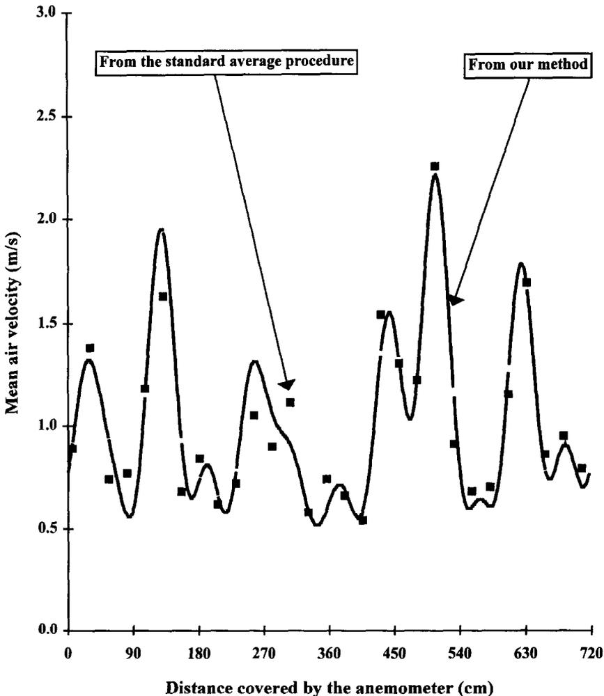
Fig. 5. Validation of the new experimental method set up in our laboratory in comparison to mean air velocities calculated from the standard average procedure.
