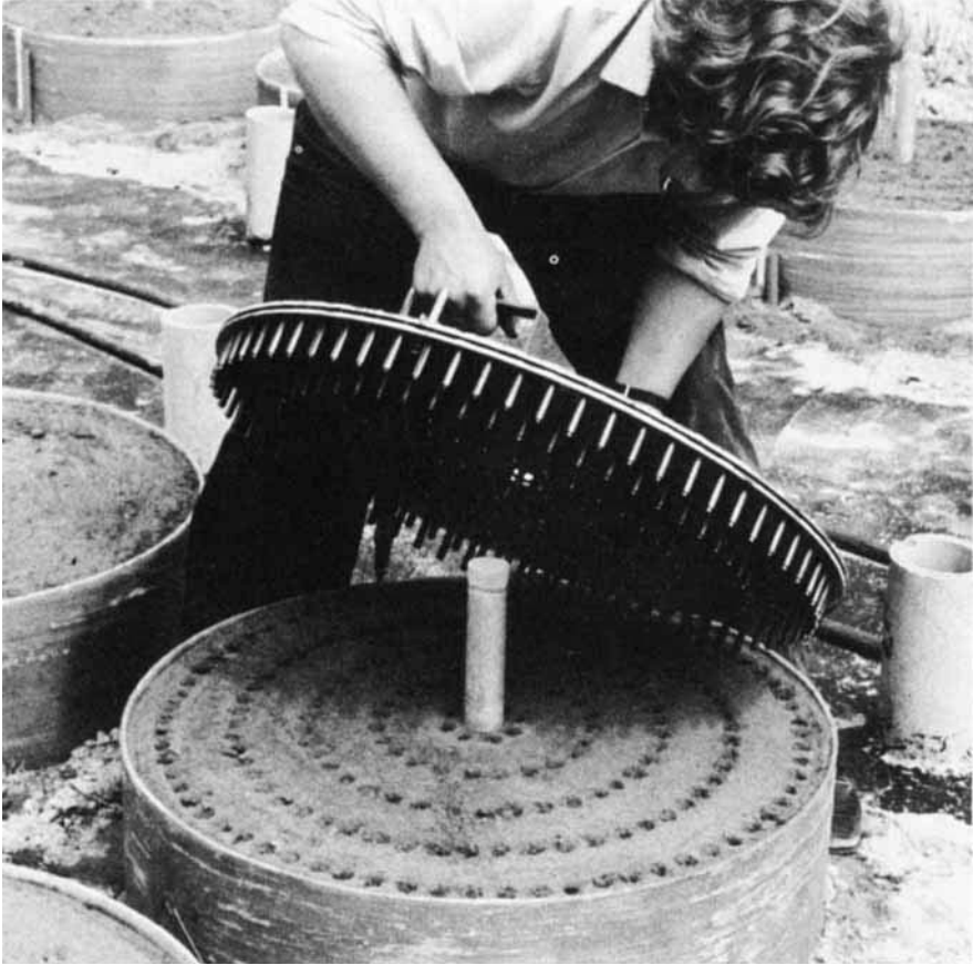
PLATE 4. Aluminium template used to sow 5 concentric rows of cereal seeds on a lysimeter. This plate can be adapted for a range of seed sizes and spacings.
