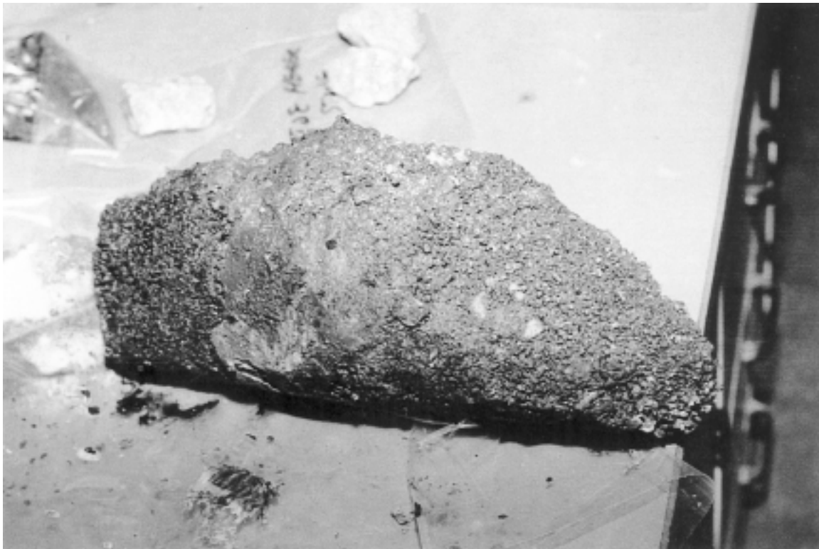
Fig. 16. Solid clog material removed from drainage pipe (this specimen has dimensions of about 100 mm wide \times 75 mm thick \times 300 mm long).
