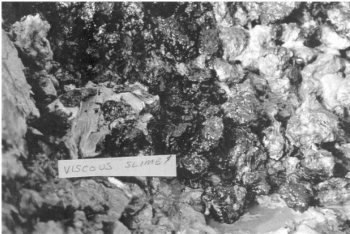
Fig. 9. Clear stone after 3 years contact with leachate.
