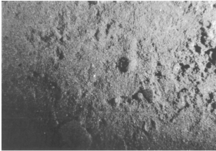
Fig. 19. Photomicrograph of bottom of clog, sample 94-12. Magnification 6 \times .
