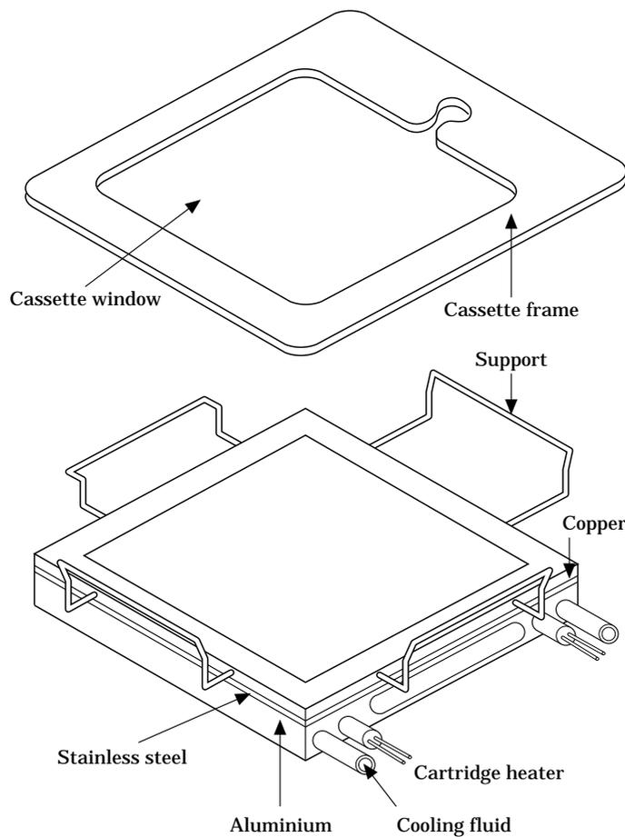
Figure 1. Schematic diagram of the gel cassette on the controlled temperature block.
