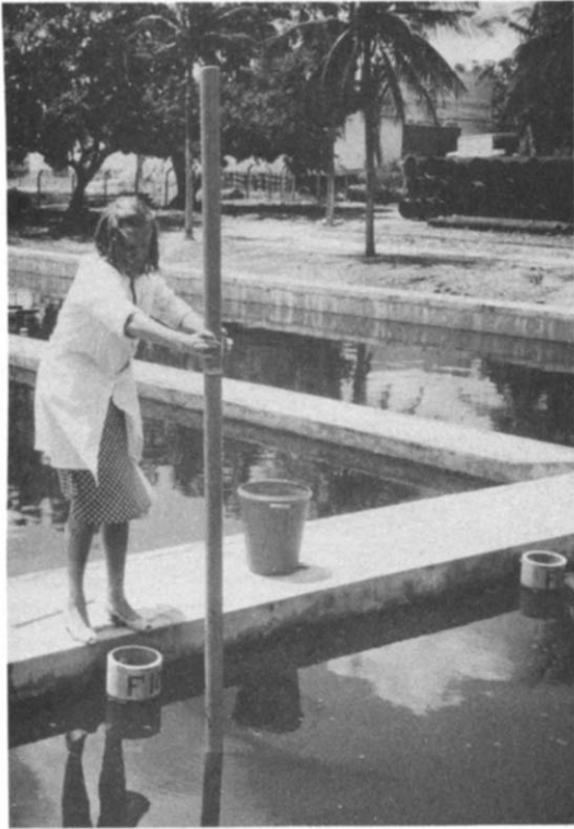
Fig. 2. A 3-m pond column sampler in use at a pilot pond in northeast Brazil.
