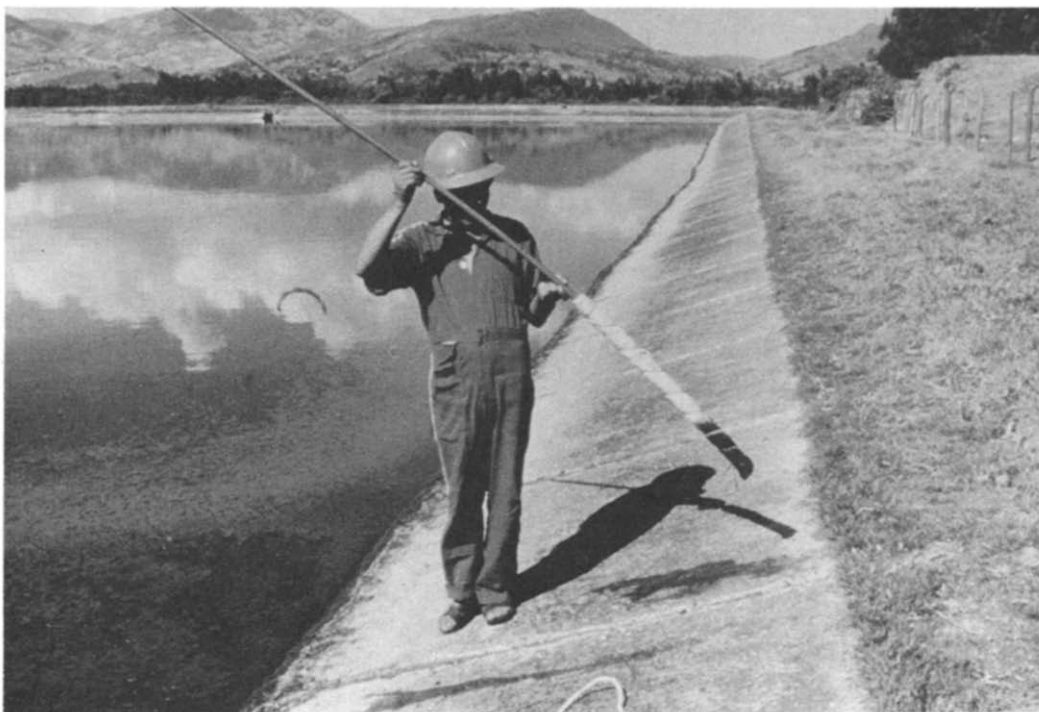
Fig. 4. Measurement of sludge depth in a facultative pond in Peru using the "white towel test".
