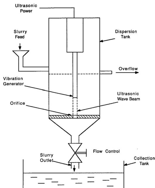
**FIGURE 1.** Schematic diagram of the apparatus for dispersing fibers.
