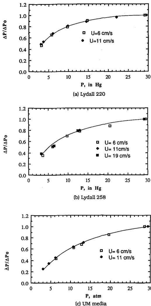
**FIGURE 7.** Normalized pressure drop,  $\Delta P/\Delta P_0$ , at different pressures ( $\Delta P_0 =$  pressure drop at 1 atm): (a) Lydall 220 medium; (b) Lydall 258 medium; (c) UM media.
