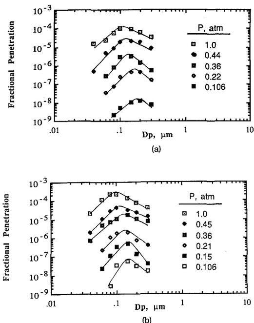
**FIGURE 6.** Fractional penetrations of the UM medium at various pressures: (a)  $U = 11$  cm/s; (b)  $U = 19$  cm/s.
