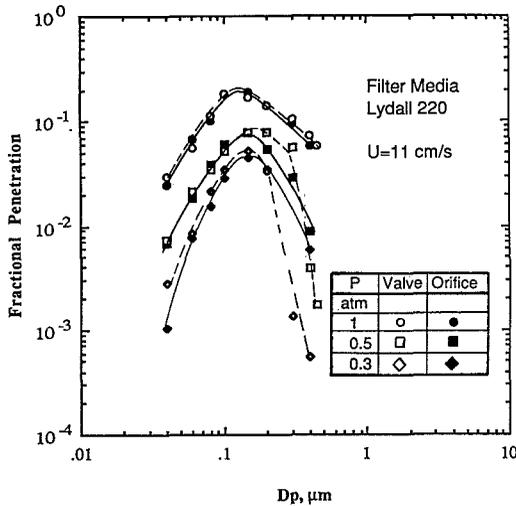
FIGURE 3. Comparisons of the penetrations obtained with the different pressure control devices.
