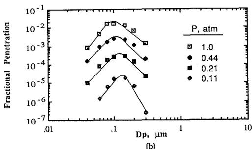
**FIGURE 4.** Fractional penetrations of the Lydall 220 medium at various pressures: (a)  $U = 6$  cm/s; (b)  $U = 11$  cm/s.
