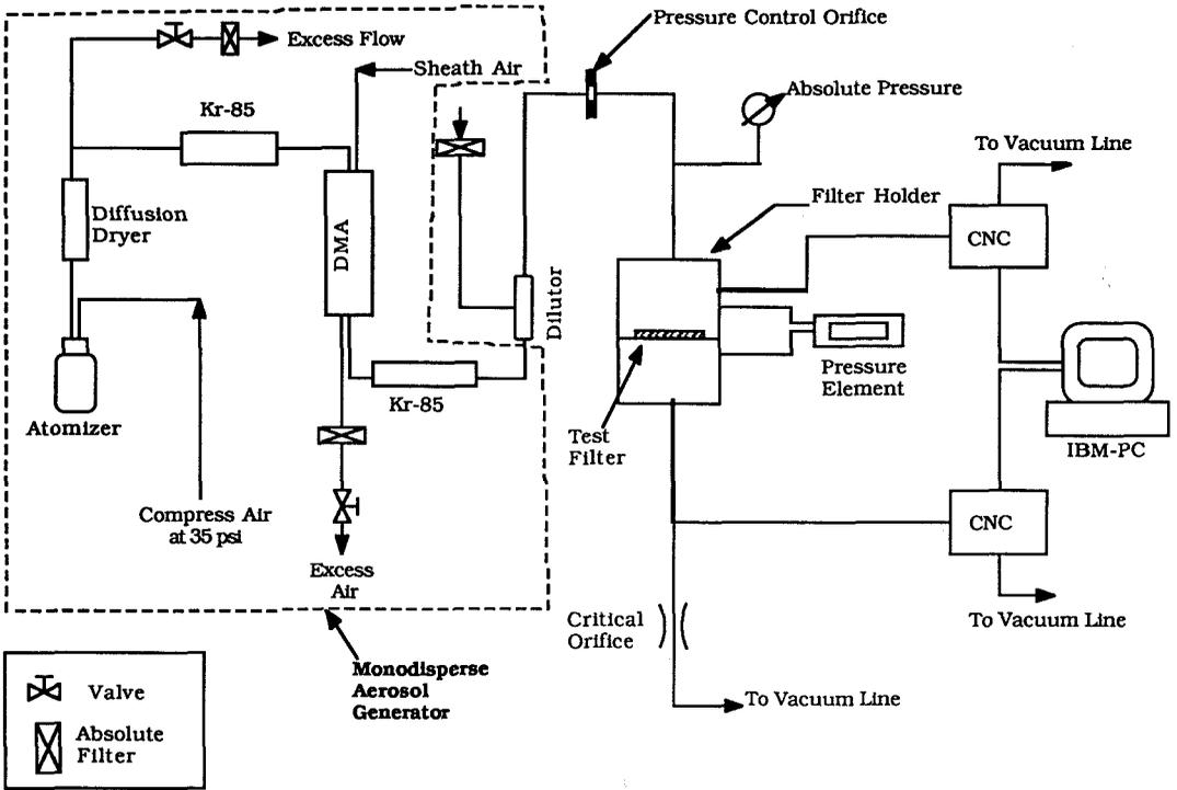
FIGURE 2. Schematic diagram of the experimental system for testing filters at reduced pressures.
