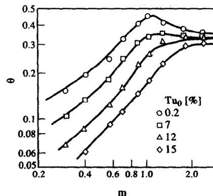
Fig. 6. Dependence of  $\Theta$  on the injection parameter  $m$ .
