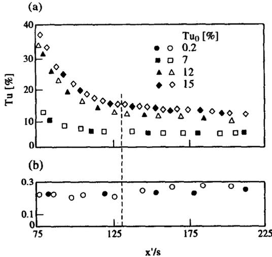
Fig. 3. Distribution of turbulence intensity with a high (a) and low (b) initial turbulence intensity along the channel axis. Light points—without jet injection, dark points—with a wall jet supply ( $m = 2$ ).
