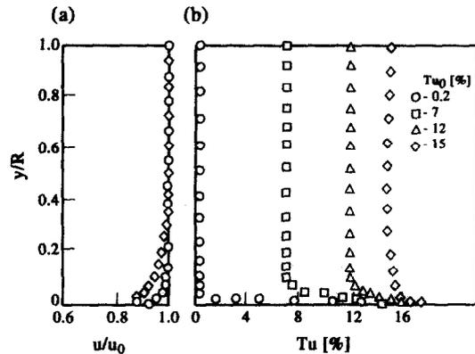
Fig. 2. Profiles of average velocity (a) and turbulence intensity (b) on the working channel inlet.
