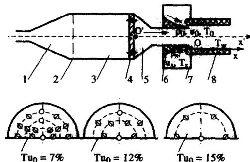
Fig. 1. Scheme of an experimental setup for investigation of cooling effectiveness in a high-turbulent flow: 1—inlet diffuser; 2—smoothing grid; 3—setting chamber; 4—turbulizing grids; 5—confusor; 6—separating slot-lip; 7—injection chamber; 8—experimental cylindrical section.
