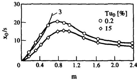
Fig. 7. Length of the initial section at different injection parameters.
