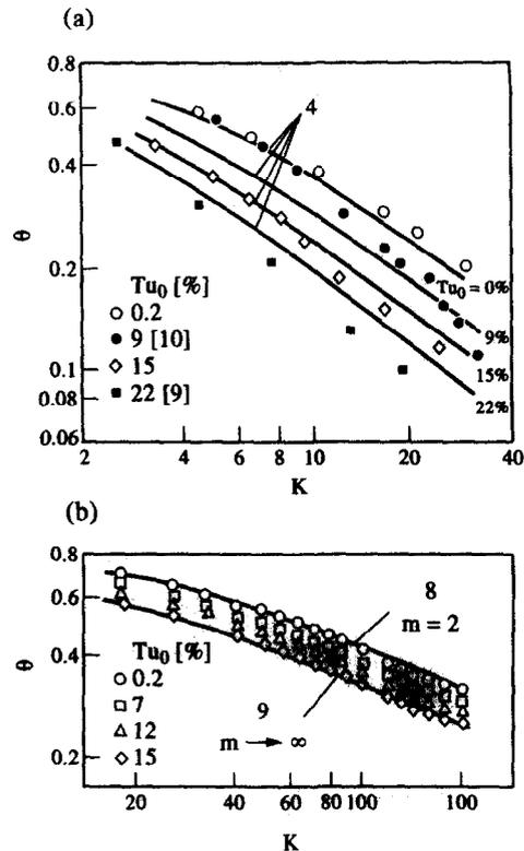
Fig. 8. Generalization of experimental data on effectiveness of high-turbulent wall cooling: (a)  $m < 1$ ; (b)  $m > 1$ .
