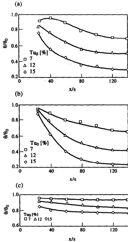
Fig. 5. Relative values of the wall jet cooling effectiveness with the initial turbulence change: (a)  $m = 0.6$ ; (b)  $m = 0.9$ ; (c)  $m = 2$ .
