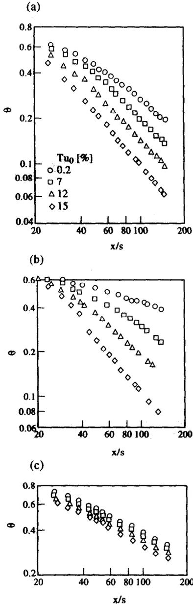
Fig. 4. Distribution of the effectiveness parameter along the channel length with different turbulence intensities and injection parameters: (a)  $m = 0.6$ ; (b)  $m = 0.9$ ; (c)  $m = 2$ .
