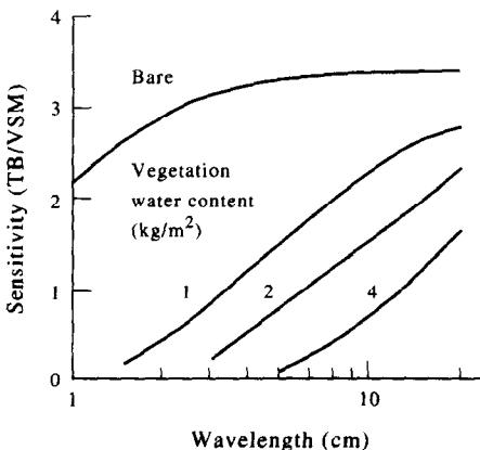
Fig. 2. Sensitivity of brightness temperature to soil moisture as a function of wavelength for bare and vegetated conditions (H polarization 10° look angle).
