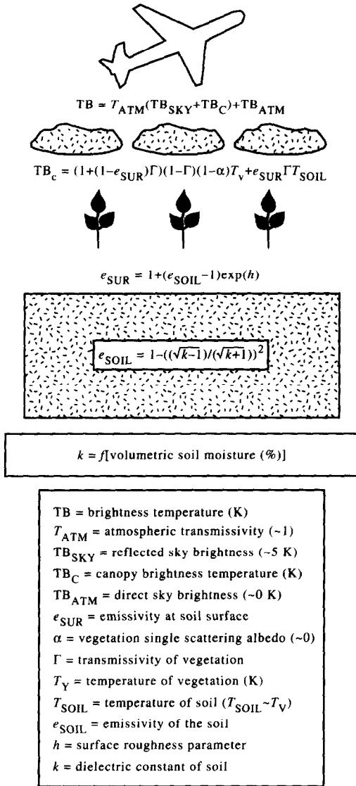
Fig. 1. Schematic of a passive microwave emission model from land surfaces.
