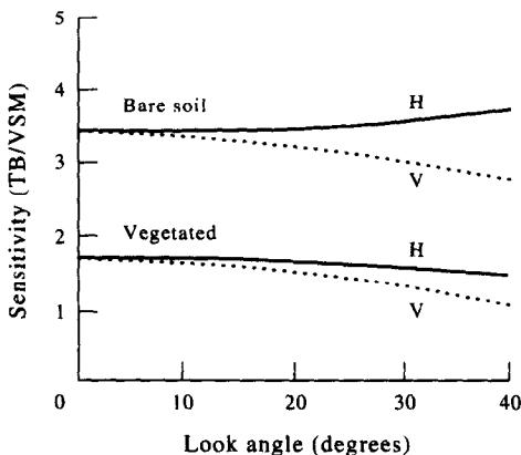
Fig. 4. Sensitivity of brightness temperature to soil moisture as a function of look angle for H and V polarizations (L band).
