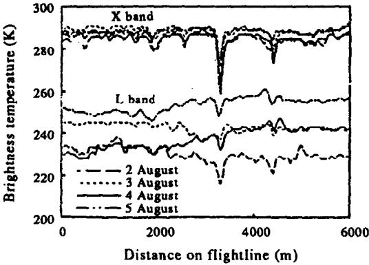
Fig. 3. Multitemporal-multifrequency aircraft radiometer observations of brightness temperature collected over the Walnut Gulch study site in August 1990[4].
