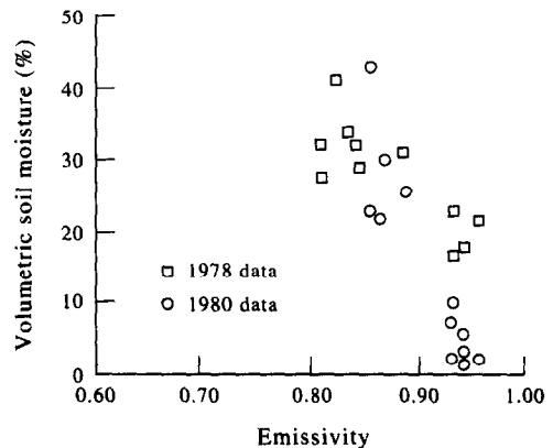
Fig. 5. Multitemporal aircraft observations of emissivity and volumetric soil moisture (0-5 cm) for rangeland sites from [5]: A-L band data and B-C band data.
