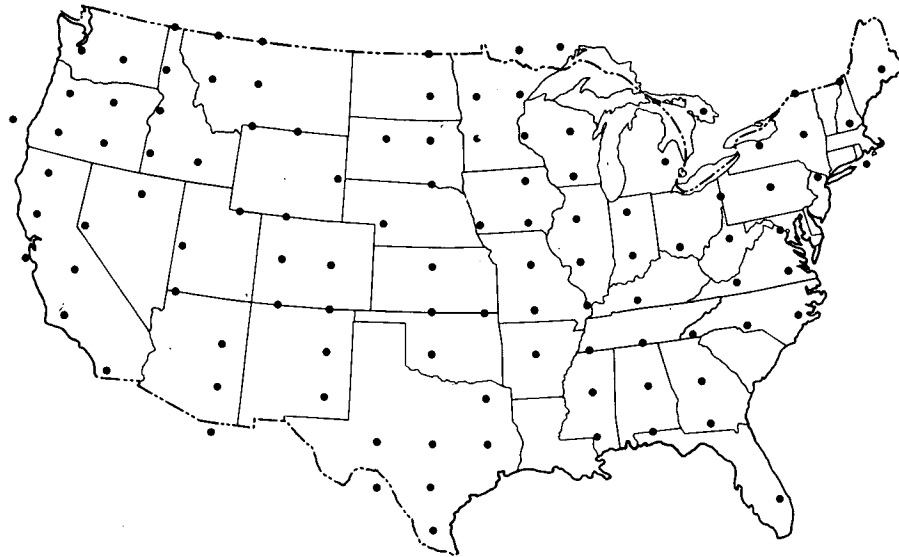
FIG. 1. Centroids of 106 2.0° lat by 3.0° long grid cells containing streamflow data used in the principal components analysis.
