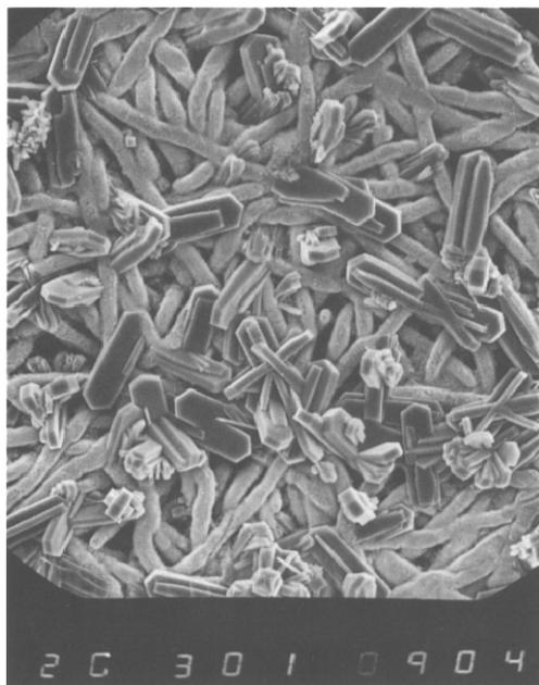
Fig. 6. SEM picture of small MFI crystals on top of a two-layer stainless steel support, prepared according to SS-2 (magnification 300 $\times$ ).
