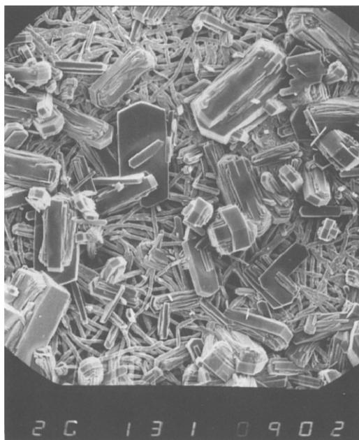
Fig. 8. SEM picture of a partly covered two-layer stainless steel support, prepared according to SS-4 (magnification 130 $\times$ ).
