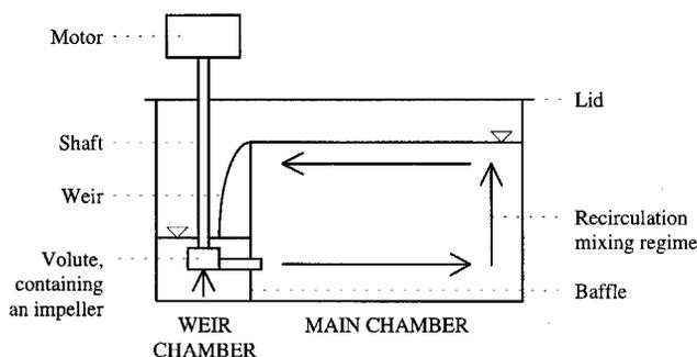
Figure 1. Schematic vertical section through the weir tank reactor.
