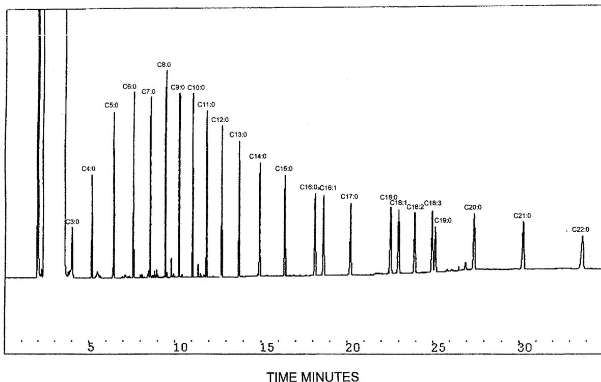
Figure 2. Gas chromatographic separation of fatty acid methyl esters derivatized with TMSH.
