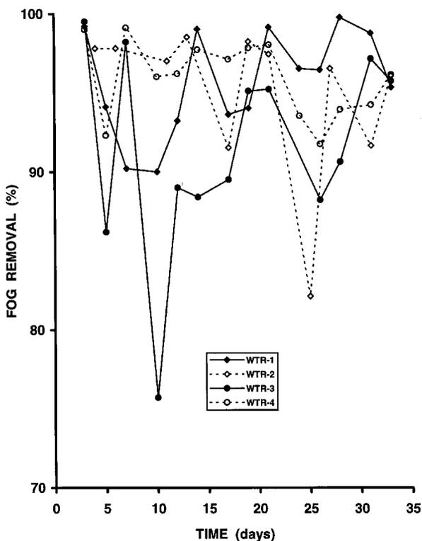
Figure 4. Bioreactor FOG removal.
