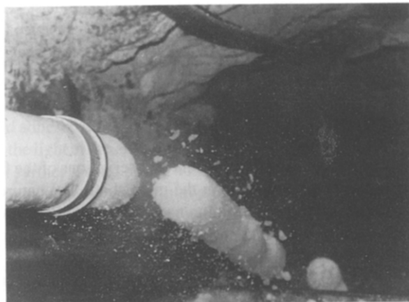
Fig. 5. Full ice plugs emerging on 42 level at an ice flow rate of 2.76 kg/s.
