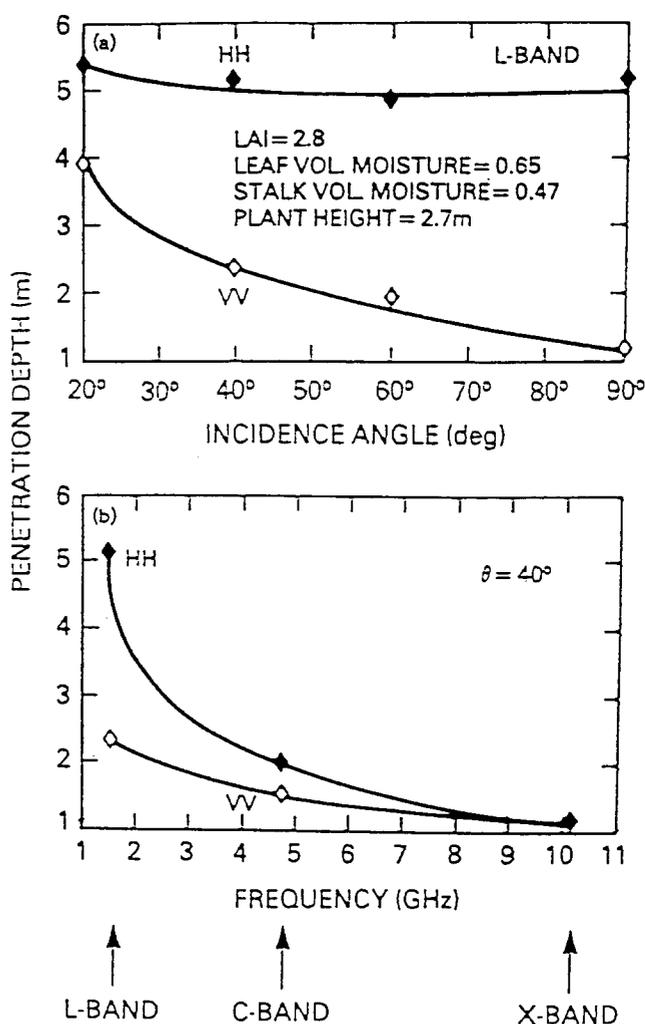
Figure 6. An illustration of the penetration depth of a corn canopy versus incidence angle for HH and VV polarization at (a) L-band, and (b) 40° (after NASA, 1988).
