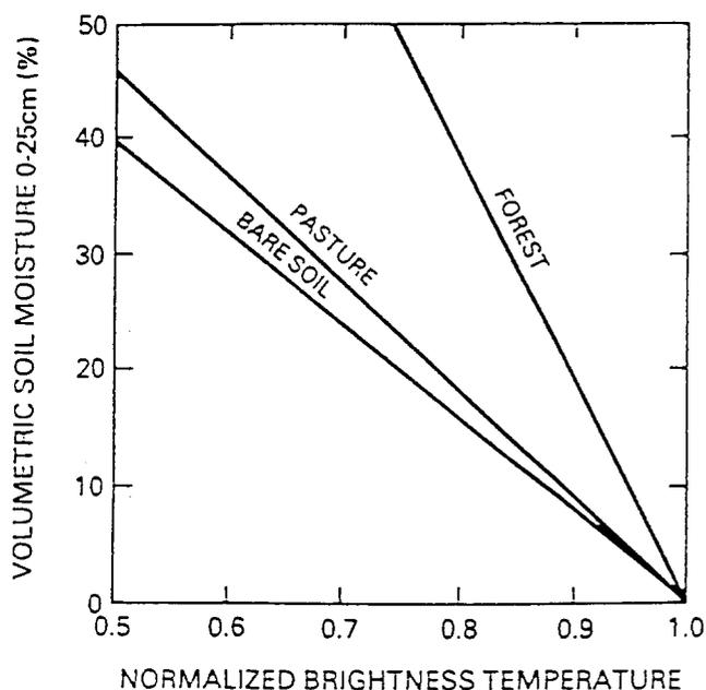
Figure 5. Relationships between normalized brightness temperature and soil moisture for bare soil and different types of vegetation; L band at HH - polarization at 10° (after Jackson et al., 1982).
