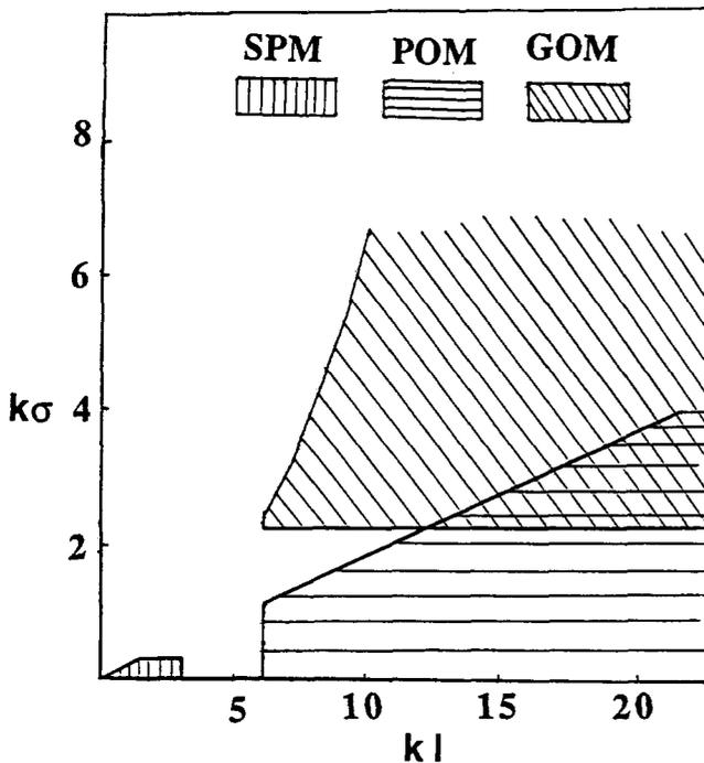
Figure 4. Regions of validity for different scattering models and roughness parameters (after Oh et al., 1992).
