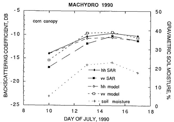
Figure 8. L-band AIRSAR data and modeling results from a corn field with varying soil moisture.
