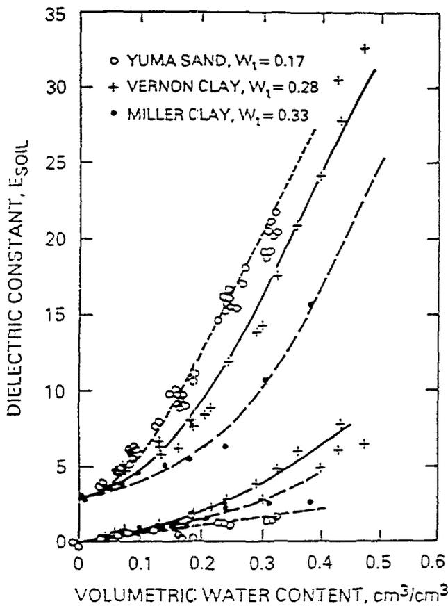
Figure 2. A comparison of laboratory measurements of the real and imaginary parts of the dielectric constant and model predictions (smooth curves) for three soils as functions of moisture content at a wavelength of 21 cm (after Wang and Schmugge, 1980).  $W_t$  denotes transition moisture.
