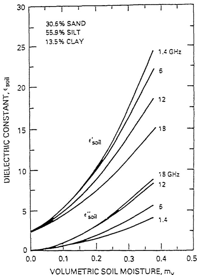
Figure 1. An illustration of the real ( $\epsilon'_{\text{soil}}$ ) and imaginary ( $\epsilon''_{\text{soil}}$ ) parts of the dielectric constant as a function of volumetric moisture content for a loamy soil measured at four frequencies (after Ulaby et al., 1986).
