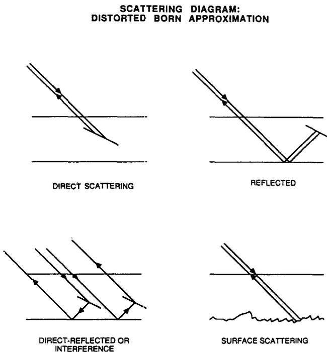
Figure 7. Dominant scattering mechanisms from a layer of vegetation.
