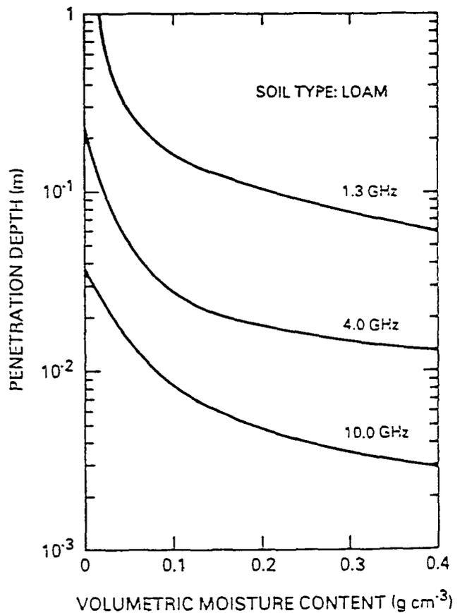
Figure 3. Penetration depth as a function of moisture content for three frequencies (after Ulaby et al., 1982).
