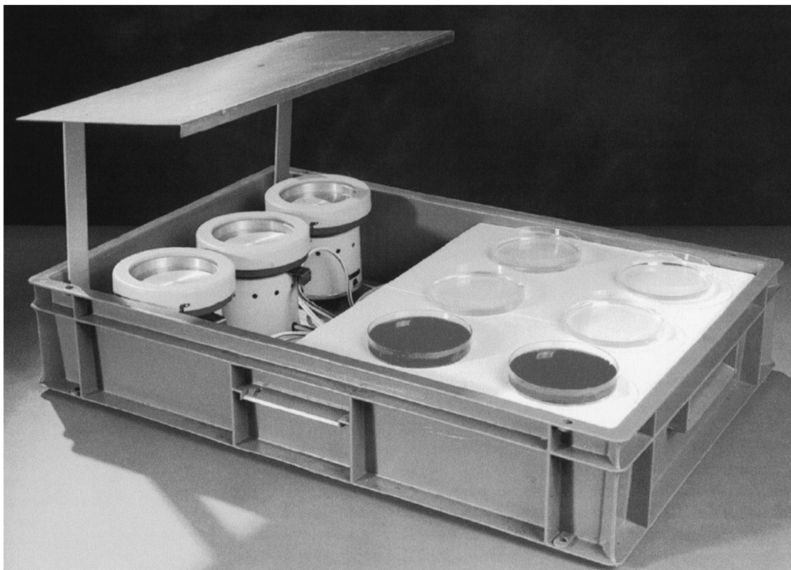
Fig. 1. Air sampling equipment. Left-hand-side shows three air samplers shielded by a pitched steel sheet. Right-hand-side shows two rows of agar plates (settle plates), one row directly below carcasses to detect organisms in drips and one not below carcasses to detect organisms in deflected water droplets.
