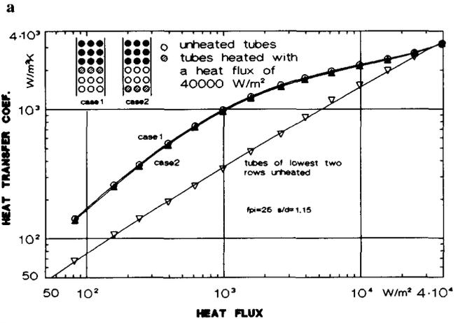
Figure 6. Effect of the position of extra heating on heat transfer.
