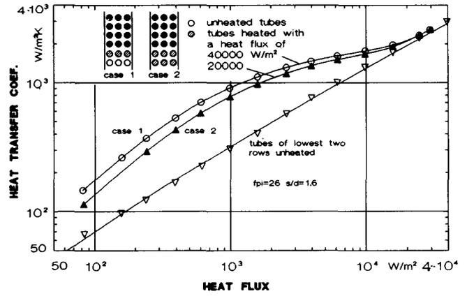
Figure 7. Effect of heat flux of extra heating on heat transfer.
