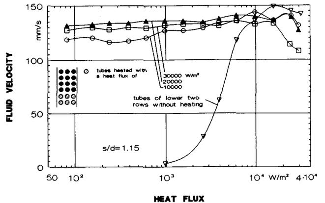
Figure 8. Fluid velocity under the bundle.
