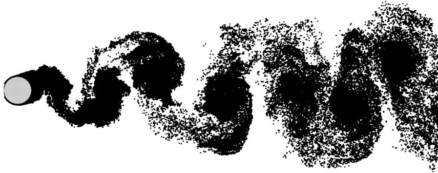
Fig. 2. Computed streaklines, von Kármán vortex street past a circular cylinder at  $Re = 140,000$ .
